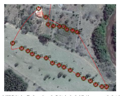
**Figure 8.** Hill flight plan. The figure shows the flight plan for the hill video sequence: the first slope is between Waypoints 1 and 16 and the second between Waypoints 19 and 25.
