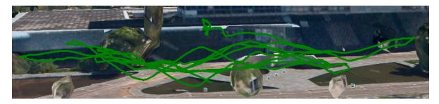
Figure 14. Manual flight path with vertical zig-zag pattern.
