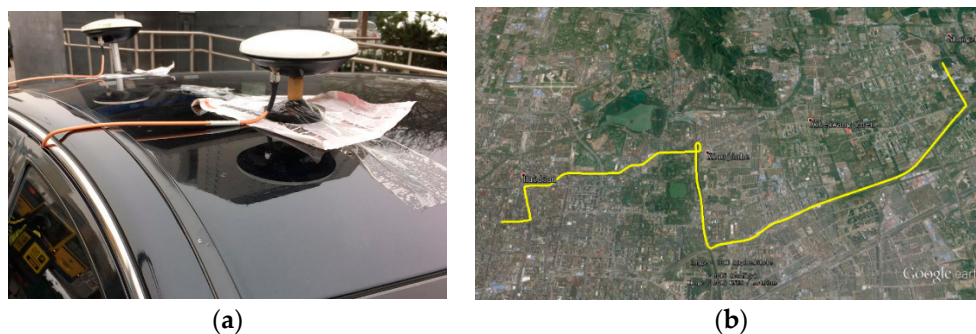
Figure 15. The urban vehicle test condition: (a) the location of two antennas; (b) the route of the urban vehicle test.
