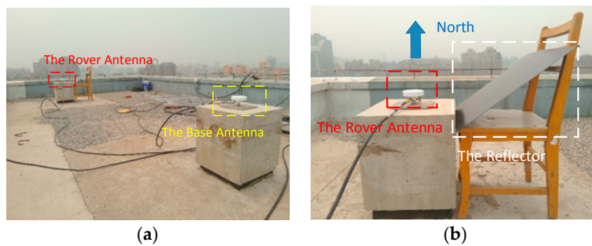
Figure 10. The multipath environment: (a) the location of the two antennas; (b) the illustration of the reflector.
