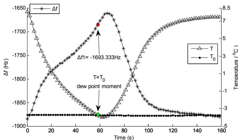
**Figure 8.** Variation regularity of  $\Delta f$  in a temperature-control circle.
