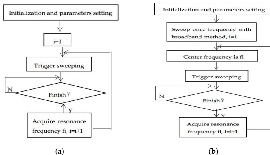
**Figure 3.** Two methods of measuring  $f_0$ : (a) the broadband method and (b) the narrow band method.
