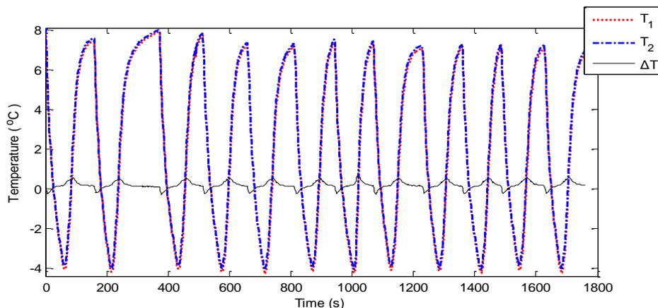
Figure 5. The measured temperature of the dual quartz crystal microbalance (DQCM).
