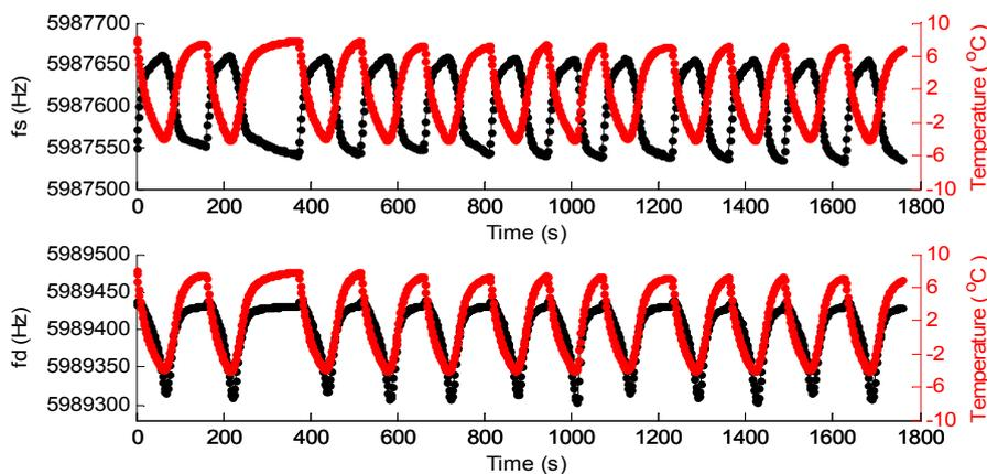
Figure 7. The frequencies of the DQCM with the change in temperature.
