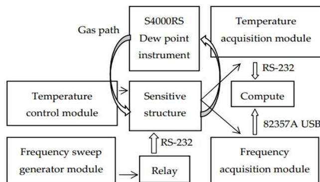
**Figure 2.** Experimental set-up.
