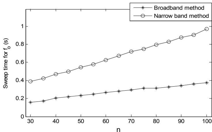
Figure 4. The relationship between  $n$  and sweep time for  $f_0$ .
