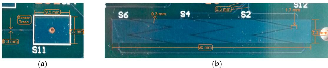
**Figure 6.** Construction of electrodes of self-capacitive (a) single sensor; (b) slider.
