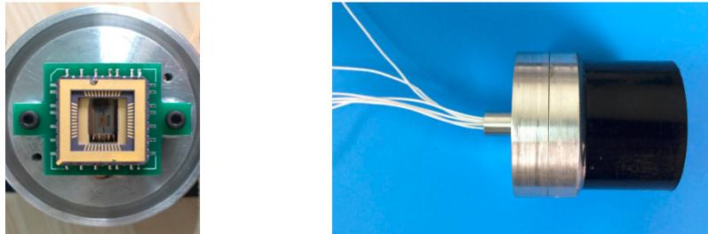
Figure 12. Prototype of the MEMS electronic heart sound sensor.
