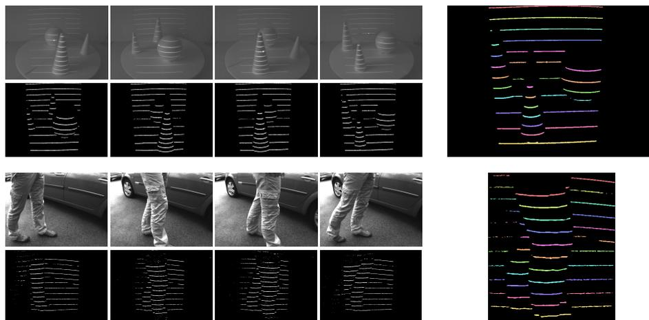
**Figure 13.** Sample images from the two datasets used in the experiments. The upper group of images shows sample images from the indoor dataset, and the lower group of images shows samples from the outdoor dataset. Both visible-spectrum and demodulated images are shown. The images on the right show the color-coded ground truth (best viewed in color).
