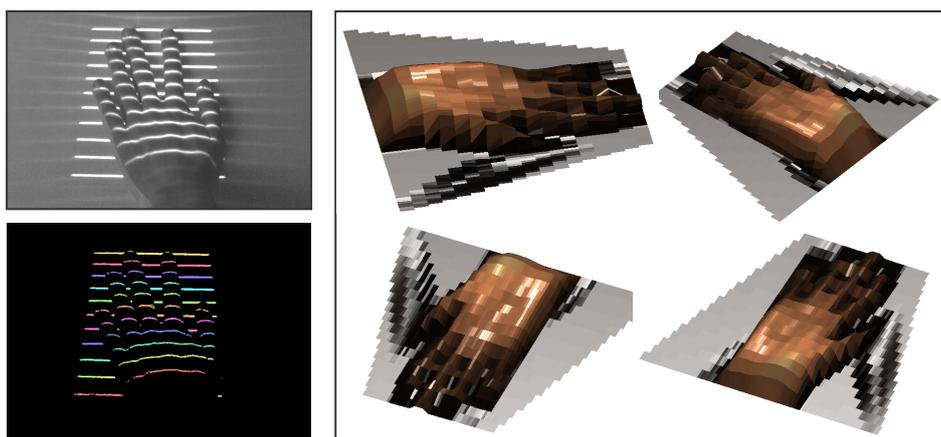
**Figure 18.** A visual example of the 3D reconstruction capabilities of the developed sensor. The image in the upper left corner shows a (visible light) image of the observed scene (i.e., a hand); the image in the lower left corner shows the labeled distortion map; and the image on the right shows the depth image from our ATRIS sensor from various viewing angles.
