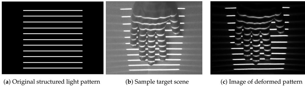
**Figure 3.** The correspondence problem: (a) an illustrative image of the structured light pattern produced by the ATRIS sensor, without distortions; (b) an example of a target scene illuminated by the light pattern; (c) an example of the spatial distortion map captured with the sensor. To be able to reconstruct a depth image of the target scene, each pixel comprising the light pattern in (c) needs to be assigned a label corresponding to one of the light planes in the pattern shown in (a).
