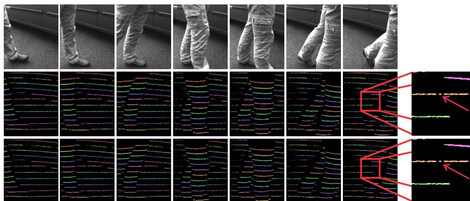
**Figure 16.** Visual examples of the results of the proposed light plane labeling procedure. The first row shows sample images from the outdoor dataset; the second row shows the (color-coded) manually-annotated ground truth; and the third row shows color-coded results of the labeling procedure. The images on the right side show an example of a labeling error, which is highlighted by arrows (best viewed in color).
