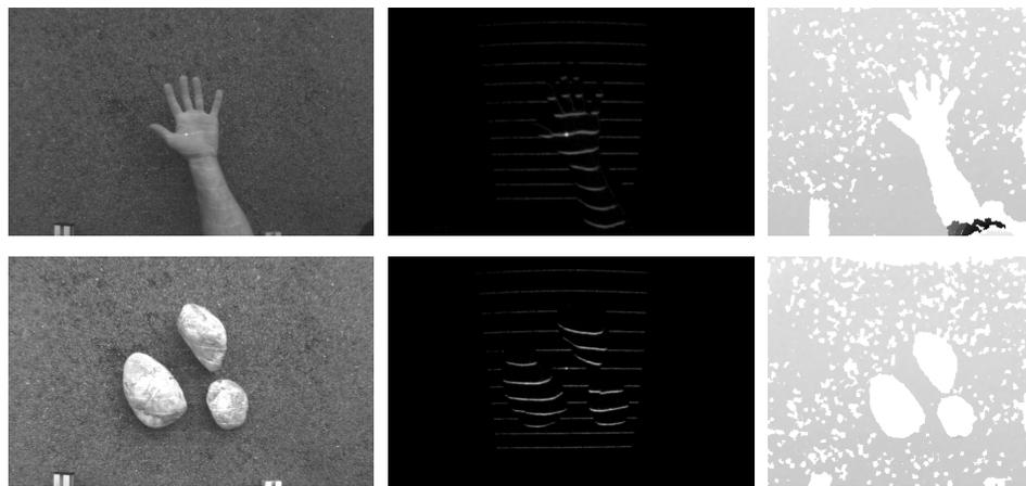
**Figure 11.** Illustrative example of the behavior of the developed acquisition procedure when deployed in outdoor environments. The first column shows gray-scale images of the target scene, the second column shows the distortion maps captured with the ATRIS sensor; and the last column of images presents the output of the Kinect sensor. The upper row presents images taken under exposure to moderate sunlight, and the lower row shows images taken under exposure to strong incident sunlight.
