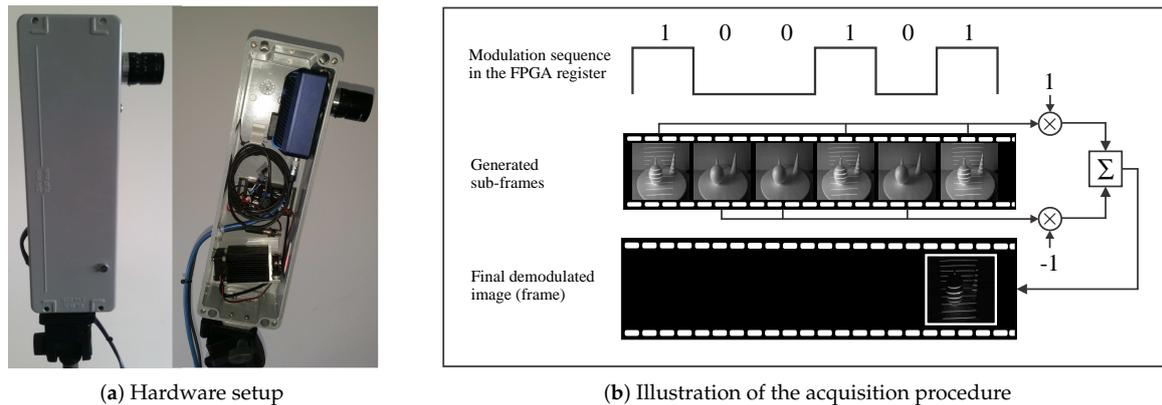
**Figure 2.** The acquisition procedure. (a) Visual appearance of the hardware setup of the ATRIS sensor. The left side of the image shows the casing of the sensor and the right side the arrangement of the camera (above) and the laser projector (below) in the casing. (b) Illustration of the modulated acquisition procedure.
