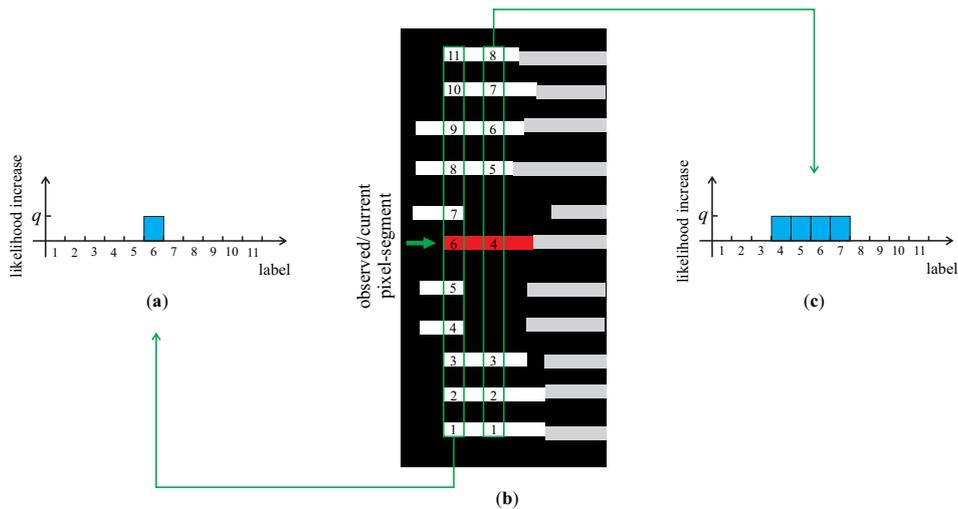
**Figure 7.** Computing prior factors: illustration of the procedure with a simple example (shown in (b)). For each random variable, the prior factor represents a probability distribution over all light-plane labels. Estimates of the probabilities are obtained by labeling the pixel segments and increasing the likelihood (shown in (a) and (c)) of the label assigned to the observed pixel segment at each  $x$ -coordinate.
