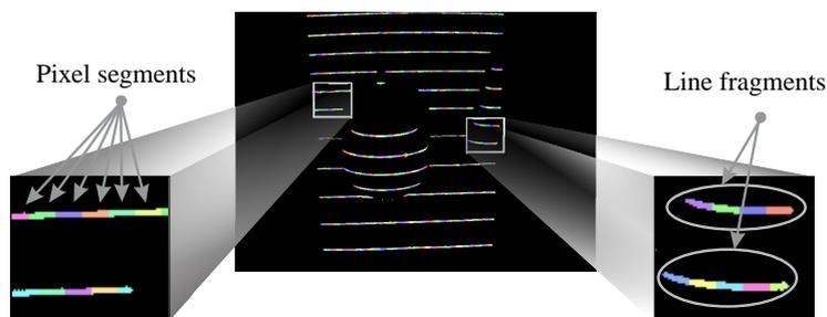
**Figure 4.** Visual illustration of some terminology used in this paper. Connected binary regions (using eight-adjacency) are referred to as line fragments. Smaller parts of the line fragments of fixed width are referred to as pixel segments.
