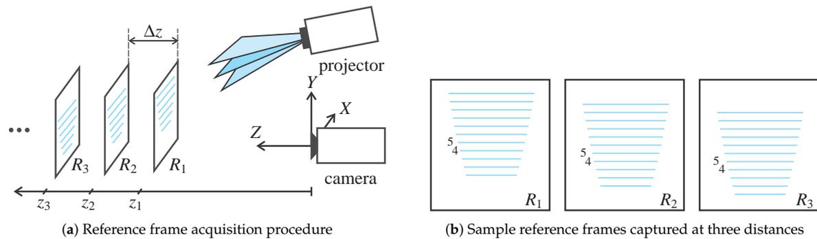
**Figure 8.** Illustration of the reference frame acquisition procedure: (a) the setup; (b) sample reference frames captured at distances  $z_1$ ,  $z_2$  and  $z_3$ . The reference frames are used to compute the depth value of each pixel segment in the labeled distortion map.
