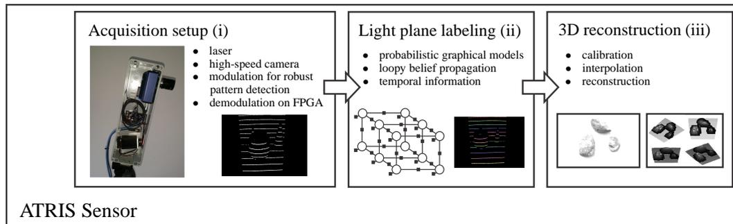
**Figure 1.** Schematic representation of our active triangulation system (ATRIS) sensor. The sensor comprises three key components: (i) an image acquisition procedure, which captures an image of the projected light pattern; (ii) a light plane labeling technique, which establishes the correspondence between all parts of the projected and detected patterns; and (iii) a 3D reconstruction procedure, which constructs a depth image from the detected light pattern.
