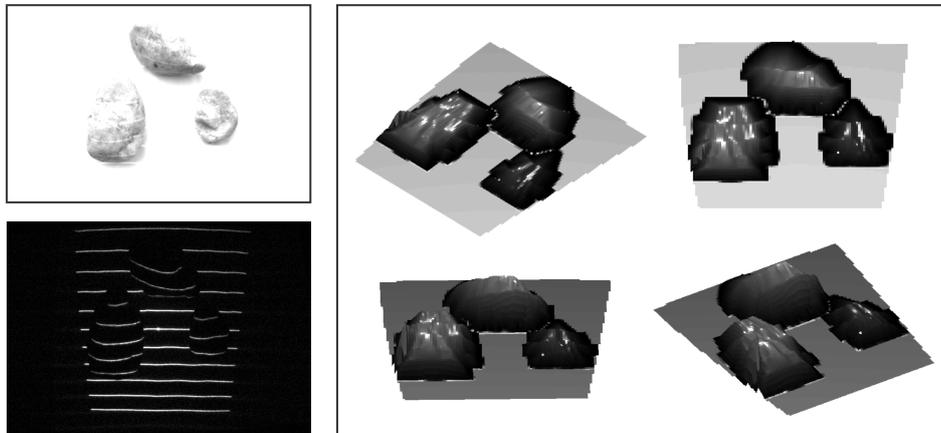
**Figure 17.** A visual example of the 3D reconstruction capabilities of the developed sensor. The image in the upper left corner shows a (visible light) image of the observed scene captured under strong incident sunlight; the image in the lower left corner shows the image of the detected light pattern; and the image on the right shows the reconstructed depth image from various angles.
