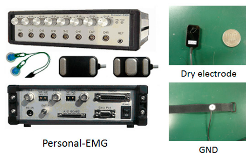
Figure 2. Experimental setup of surface electromyography (sEMG) acquisition.
