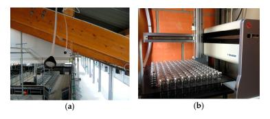
**Figure 2.** (a) The sampling point at the leeward side of the barn to measure gas concentrations. (b) The offline system (Gilson, GX-271 sampler) with evacuated glass vials.
