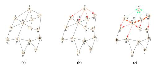
Figure 5. Signaling process: Steps 1, 2 and 3. (a) Initial network; (b) Step 2; (c) Step 3.
