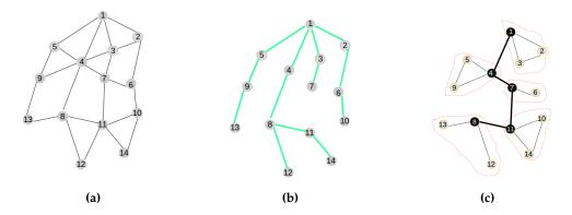
**Figure 4.** The hybrid traffic engineering model. (a) Initial network; (b) The signaling tree; (c) The clustered topology.
