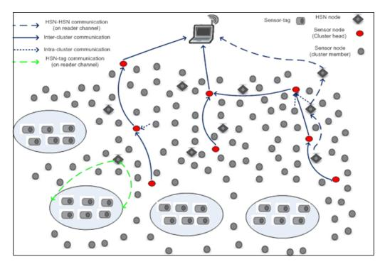
Figure 1. The hybrid Internet-of-Things model. HSN, hybrid sensor node.
