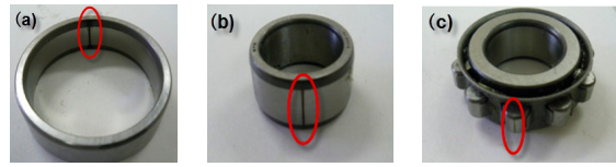
Figure 7. Bearing defects: (a) outer-race defect; (b) inner-race defect; and (c) roller defect.
