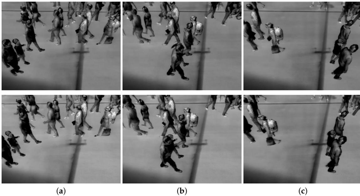
**Figure 3.** Example of pedestrians occluding each other. The upper row displays left camera images, while the bottom row displays right camera images. (a) is frame 0, (b) is frame 45, and (c) is frame 90. Note the two people entering the lower left side of the images in (a); in (b) the child is almost fully occluded, while she appears again in (c).
