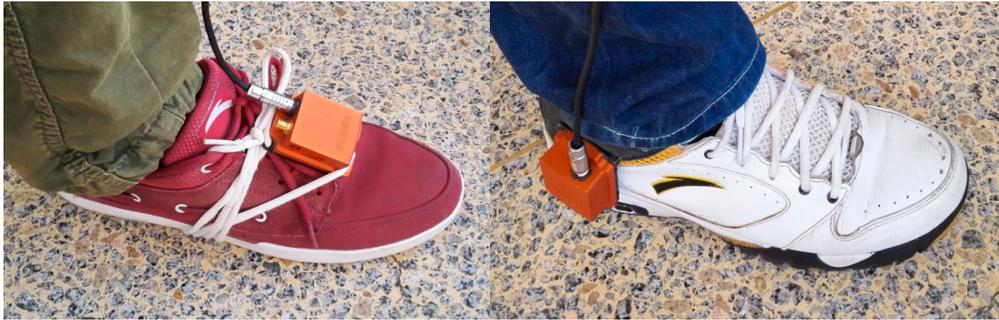
**Figure 7.** (Left) IMU strapped on the front of a shoe; (Right) IMU strapped on the rear side of a shoe.
