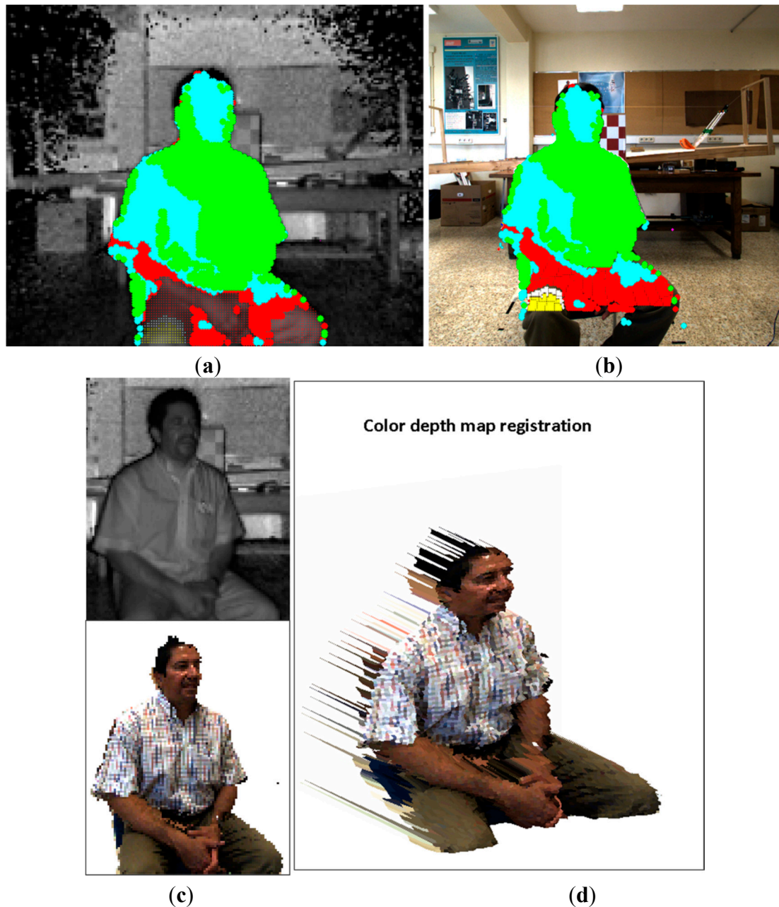
Figure 14. Image sample 33. (a) Selected points on the ToF; (b) estimated points on the RGB image; (c) Top: selected ToF ROI. Bottom: estimated RGB ROI; (d) the colour depth map of the ROI.
