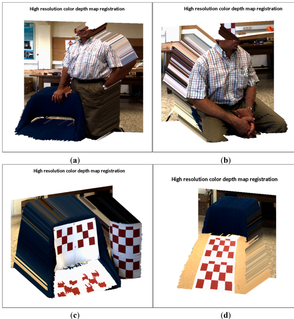
Figure 17. High resolution colour depth map reconstruction. (a) two volumetric objects placed at different distances from the sensory system; (b) an object with a large relief; (c) two curved objects; (d) a continuous surface which is slanted with respect to the cameras axis.
