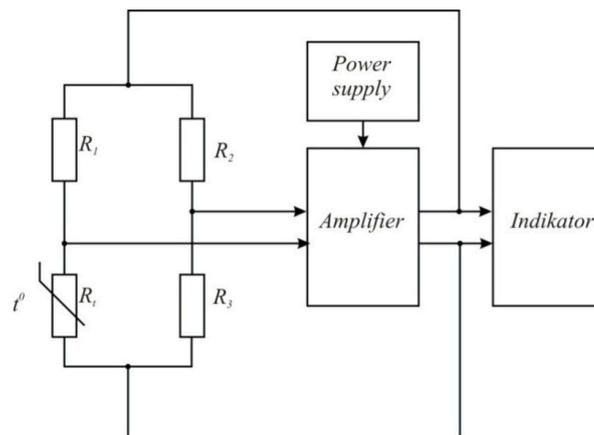
**Figure 2.** Thermo-anemometer of constant temperature type block diagram ( $t^0$ —the measured temperature).
