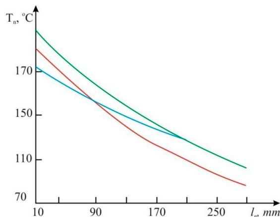
**Figure 10.** The graphs of dependence  $T_n$  on  $l_n$  ( $d_{mp}=15$  mm;  $d_n=3$  mm): — gasoline; — diesel fuel; — biofuels, the thermocouple error is 5 °C.
