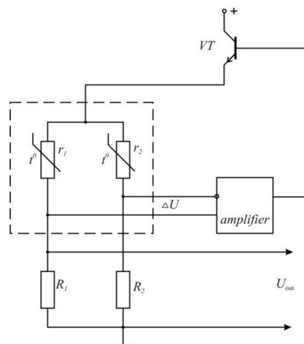
**Figure 6.** The thermo-anemometer electric circuit.
