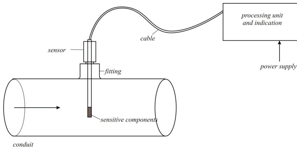
**Figure 7.** The thermo-anemometric flowmeter schematic diagram.
