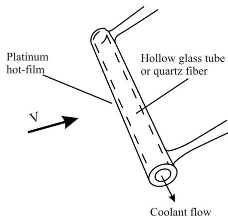
**Figure 4.** Tube thermo-anemometer diagram [10].
