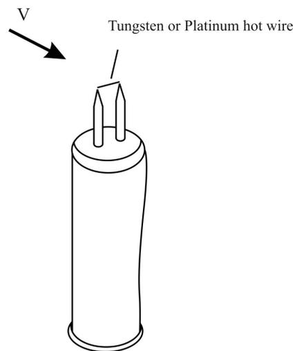
**Figure 3.** Typical thermo-anemometer diagram [10].
