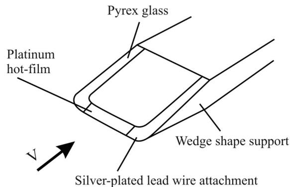
**Figure 5.** Wedge thin-film thermo-anemometer diagram [10].
