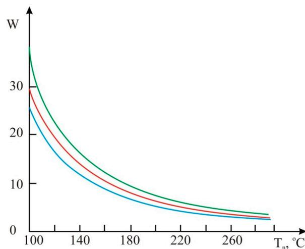
**Figure 9.** The graphs of fuel consumption dependence on heater temperature: — gasoline; — diesel fuel; — biofuels.
