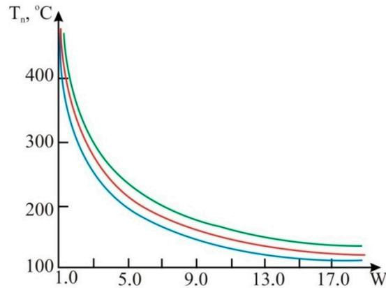
**Figure 8.** The graphs of temperature dependence on fuel consumption: — gasoline; — diesel fuel; — biofuels  $T_n, ^\circ\text{C}$ .
