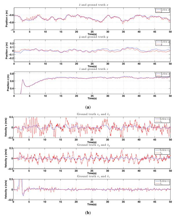
**Figure 28.** Experimental results for outdoor (night) PBVS-based hovering: estimator performance. Estimated angles are omitted and all states are shown at the same scale. The performance evaluation summary of these plots is presented in Figure 22. (a) Position estimation (red) with ground truth (blue). Note that z-axis is inverted for visualization; (b) Velocity estimation (red) with ground truth (blue),  $\hat{w}\hat{x}$ ,  $\hat{w}\hat{y}$  and  $\hat{w}\hat{z}$ .
