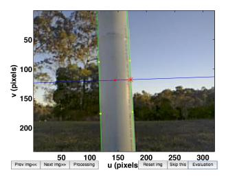
**Figure 37.** User interface of tool for generating performance metrics. The four yellow points are manually picked to define the pole edges (two green lines). The red point and star denote the calculated pole centre and width in the image coordinates respectively.
