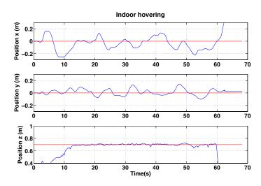
**Figure 30.** Experimental results for IBVS-based hovering: control performance for indoor IBVS-based hovering. Goal positions shown in red.
