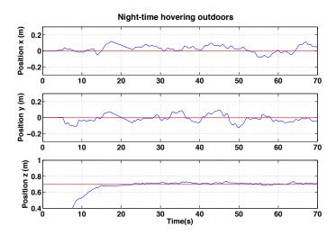
**Figure 32.** Experimental results for IBVS-based hovering: control performance for night-time IBVS-based hovering. Goal positions shown in red.
