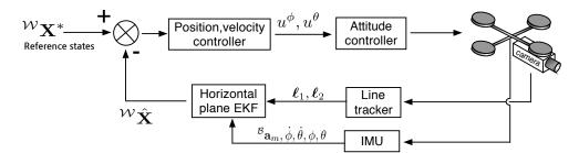
**Figure 6.** Block diagram of horizontal plane state estimator and control used for the PBVS approach.  $u^{\phi}$  and  $u^{\theta}$  denote control inputs for roll and pitch commands.  $\ell_1$  and  $\ell_2$  are tracked 2D lines and  ${}^{\mathcal{B}}\mathbf{a}_m$  is onboard inertial measurement unit (IMU) acceleration measurement.
