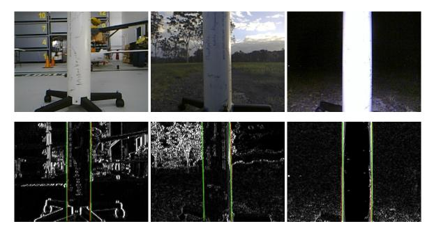
**Figure 18.** Sample onboard images from the three hovering test environments: indoor (**left**), day-time outdoor (**mid**) and night-time outdoor (**right**) respectively. The top row contains the raw images while the bottom row contains the corresponding gradient images with overlaid lines corresponding to the goal line positions (green) and the tracked pole edges (red).
