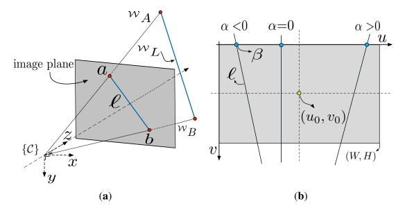
**Figure 3.** (a) Perspective image of a line  ${}^{\mathcal{W}}L$  in 3D space. *a* and *b* are projections of the world point and  $\ell$  is a line on the image plane; (b) Image plane representation of slope ( $\alpha$ ) and intercept ( $\beta$ ).
