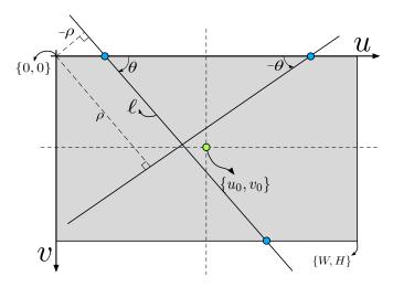
**Figure 12.** An example of the  $(\rho - \theta)$  representation for two lines,  $\ell$ . Signs of the two parameters,  $\rho$  and  $\theta$ , are shown for the corresponding positive or negative quantities.  $\{u_0, v_0\}$  is the principle point and  $\{W, H\}$  denotes the width and the height of the image plane. The origin of the pixel coordinate frame is at the top-left of the image plane by convention.
