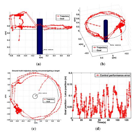
**Figure 34.** Different views of ground truth trajectory with respect to  $\{T\}$  for a pole inspection flight (**a**–**c**); (**d**) is control performance error plot, *i.e.*, 3D Euclidian distance error between the goal and the trajectory. An operator only commands yaw rate using the RC transmitter during the experiment. The constant height, 0.7 m is maintained by the system.
