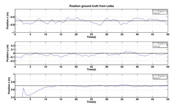
**Figure 27.** Experimental results for outdoor (night) PBVS-based hovering: control performance. Goal (black) and ground truth states (blue). The desired position for  ${}^{W}\hat{x}$ ,  ${}^{W}\hat{y}$  and  ${}^{W}\hat{z}$  is -0.7 m, 0 m and 0.7 m. We compute standard deviations of errors for each state over the interval 10 s~50 s.  $\sigma_x = 0.047 \text{ m}$ ,  $\sigma_y = 0.043 \text{ m}$ , and  $\sigma_z = 0.016 \text{ m}$ .
