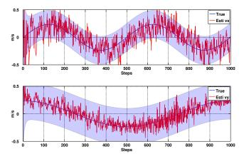
**Figure 9.** Simulation results for PBVS tracking: velocity estimation.  ${}^{\mathcal{W}}\hat{x}$  and  ${}^{\mathcal{W}}\hat{y}$  with  $3\sigma$  confidence boundary.
