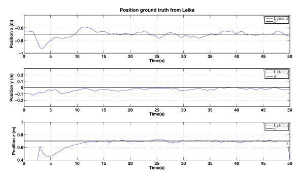
**Figure 25.** Experimental results for outdoor (day) PBVS-based hovering: control performance. Goal (black) and ground truth states (blue). The desired position for  ${}^{\mathcal{W}}\hat{x}$ ,  ${}^{\mathcal{W}}\hat{y}$  and  ${}^{\mathcal{W}}\hat{z}$  is -0.7 m, 0 m and 0.7 m. We compute standard deviations of errors for each state over the interval 10 s~50 s:  $\sigma_x = 0.038 \text{ m}$ ,  $\sigma_y = 0.028 \text{ m}$ , and  $\sigma_z = 0.022 \text{ m}$ .
