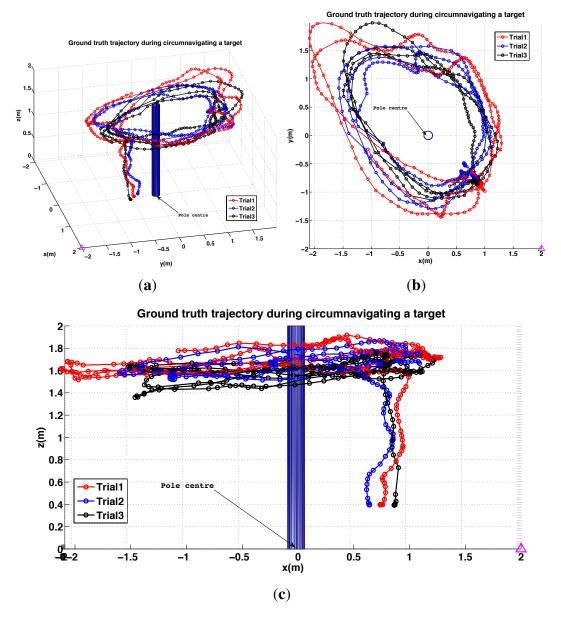
Figure 40. Experimental results for Pilot 2 during manual circumnavigation, 3D views. The magenta triangle indicates where the pilot was standing. (a) Perspective view; (b) Top view; (c) Side view.
