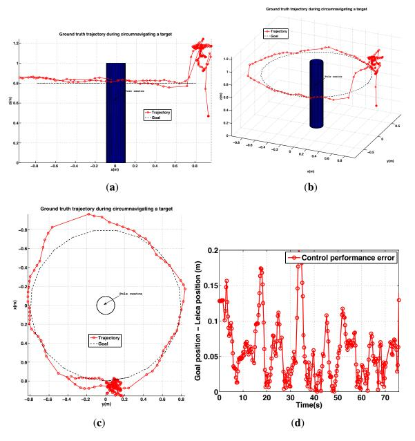
**Figure 29.** Experimental results for outdoor (day) PBVS-based circumnavigation: control performance. (**a**–**c**) 3D views of the trajectory: Side view, Perspective view and Top view; (**d**) Euclidean error (goal minus actual) trajectory *versus* time.
