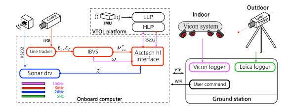
**Figure 21.** Sensor and software system diagram for IBVS experiments. Different colors denote different sampling rates. All software is implemented using a Robot Operating System (ROS). Note that only one ground truth source is used at time. The Vicon system is used for indoor ground truth while the Leica laser tracker is used outdoors.
