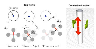
Figure 16. (left) illustration of how vehicle induces yaw motion.  $\gamma$  is an angle for the yaw motion and  $d_x$  and  $d_y$  are distances between the pole and the robot in x-, and y-axis; (right) reduced dimension task space for operator commands which is sufficient for inspection purposes.
