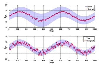
Figure 10. Simulation results for PBVS tracking: angle estimation.  $\hat{\phi}$  and  $\hat{\theta}$  with  $3\sigma$  confidence boundary.
