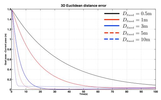
**Figure 15.** Simulation results for IBVS regulation: error response as a function of time for different assumed constant target object depths.
