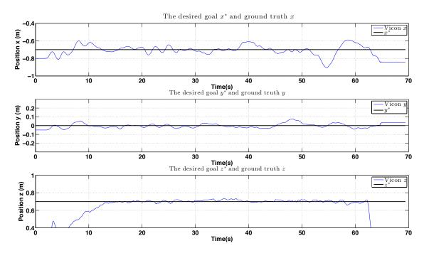
**Figure 23.** Experimental results for PBVS-based indoor hovering: control performance. Goal (black) and ground truth states (blue). The desired position for  ${}^{\mathcal{W}}\hat{x}$ ,  ${}^{\mathcal{W}}\hat{y}$  and  ${}^{\mathcal{W}}\hat{z}$  is -0.7 m, 0 m and 0.7 m. We compute standard deviation of errors for each state over the interval 15 s~63 s:  $\sigma_x = 0.048 \text{ m}$ ,  $\sigma_y = 0.024 \text{ m}$ , and  $\sigma_z = 0.011 \text{ m}$ .
