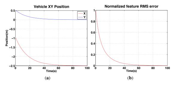
Figure 14. Simulation results for IBVS (with de-rotation): position response. (a): vehicle position (x, y) versus time showing the vehicle achieves its goal (x = -2.5, y = 0) at around 60 s; (b) the normalized root mean squared feature error  $(\ell^* - \ell)$  for the same period.
