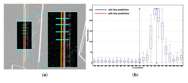
Figure 4. (a) The image at time k is shown with the tracked line from time k - 1 (without prediction case in yellow) and the predicted line from time k - 1 (with prediction case in red). We search for maxima along 60 horizontal search lines (cyan), and each is 24 pixels wide; (b) The predicted line is close to the maxima whereas there is 4.5 pixel offset without prediction.
