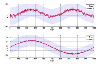
**Figure 8.** Simulation results for Position Based Visual Servoing (PBVS) tracking: position estimation.  ${}^{\mathcal{W}}\hat{x}$  and  ${}^{\mathcal{W}}\hat{y}$  with  $3\sigma$  confidence boundary.
