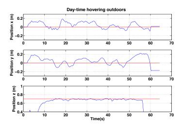
**Figure 31.** Experimental results for IBVS-based hovering: control performance for outdoor day-time IBVS-based hovering. Goal positions shown in red.
