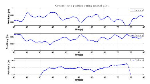
Figure 36. Experimental results for Pilot 2 during manual hovering: position versus time.
