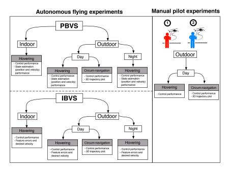
**Figure 17.** Overview of experiments. There are two categories: autonomous flying with shared autonomy (**left**) and manual piloting with only attitude stabilization (**right**); Autonomous flying consists of PBVS (**top**) and IBVS (**bottom**). Two pilots were involved in the manual piloting experiments. Each box with grey denotes a sub-experiment and describes key characteristics of that experiment.
