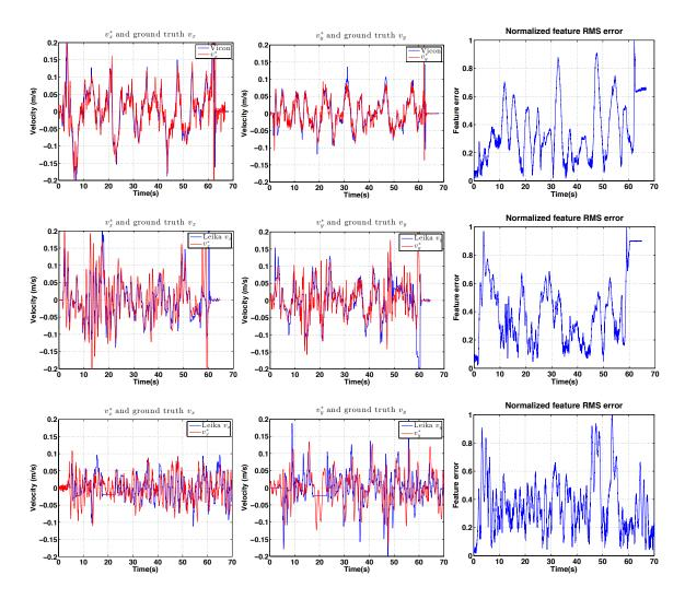
Figure 33. Experimental results for IBVS-based hovering: control demand.  $v_x^*$  (left column) and  $v_y^*$  (middle column) compared to ground truth. The first row is for indoor hovering while the second and the third rows are for day and night-time outdoor hovering. Normalized root mean squared (RMS) image feature errors for each are shown in the (right column).
