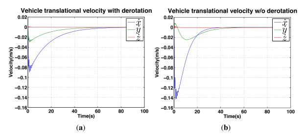
Figure 13. Simulation results for IBVS regulation: velocity response. (a) with de-rotation; (b) without.
