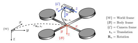
**Figure 2.** Coordinate systems: body  $\{\mathcal{B}\}$ , world  $\{\mathcal{W}\}$ , and camera  $\{\mathcal{C}\}$ . Transformation between  $\{\mathcal{B}\}$  and  $\{\mathcal{C}\}$  is constant whereas  $\{\mathcal{B}\}$  varies as the quadrotor moves.  ${}^{\mathcal{C}}\mathbf{R}_{\mathcal{B}}$  rotates a vector defined with respect to  $\{\mathcal{B}\}$  to a vector with respect to  $\{\mathcal{C}\}$ .
