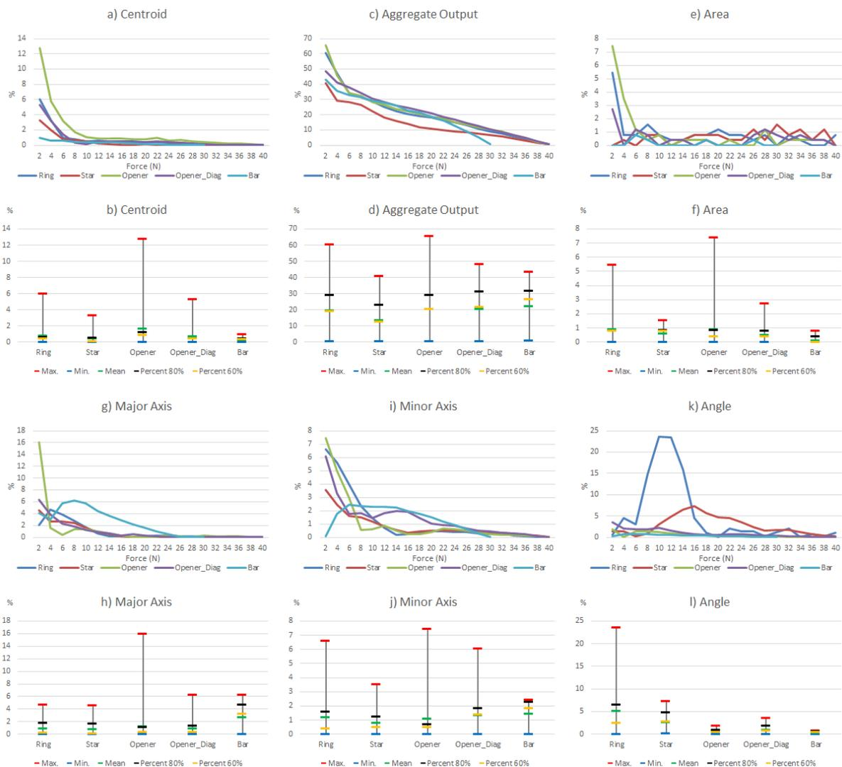
**Figure 6.** Variations of the system level parameters caused by the PCB based sensor hysteresis.
