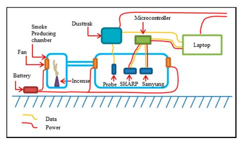
Figure 6. Gas chamber for sensor testing and calibration.
