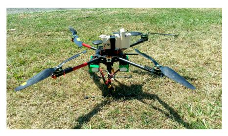
Figure 5. Quadcopter and modular gas-sensor system integrated.
