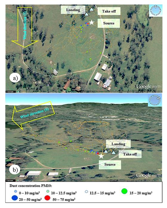
**Figure 13.** 3D visualization of Test 2 data collected with Teklite-SHARP sensor for PM10 (a) Overview and (b) Side view.
