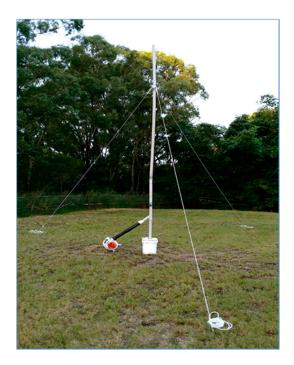
Figure 14. Powder ejection system setup.
