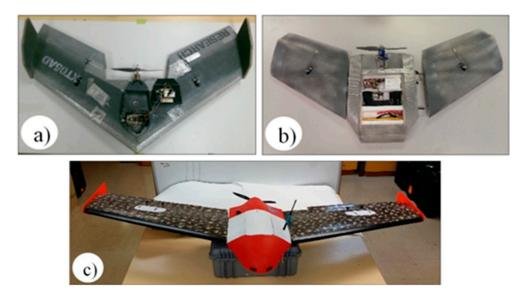
Figure 4. Fixed-wing UAV platforms, (a) Teklite; (b) GoSurv; and (c) Swamp Fox.
