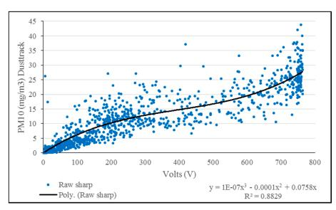
**Figure 15.** Correlation between talcum powder particles and raw value readings from the SHARP sensor and Dusttrak.
