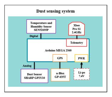
Figure 3. System architecture for the modular dust sensor.
