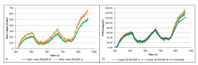
Figure 9. Dual SHARP and Dusttrak test showing (a) raw values data and (b) corrected particle measurements against Dusttrak readings.
