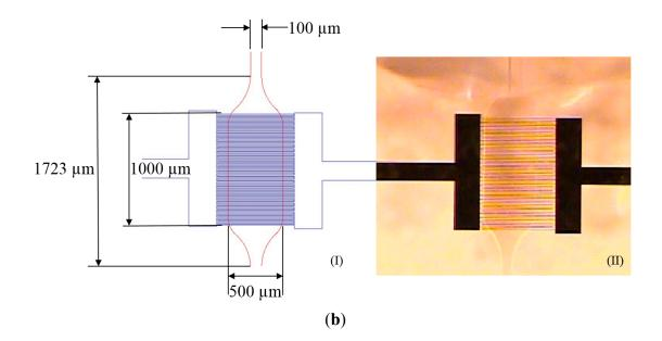
**Figure S1.** (a) Microfluidic chip with inlet port and embedded interdigitated microelectrode; (b) Gold interdigitated array microelectrode (I) drawing and (II) picture. The microfluidic channel is 40  $\mu$ m deep and 100  $\mu$ m wide with an oval-shaped microfluidics chamber (40  $\mu$ m deep, 500  $\mu$ m wide, and 1723  $\mu$ m long; 34.5 nl volume). Each electrode consisted of 25 pairs of 10  $\mu$ m wide electrode fingers spaced 10  $\mu$ m apart.
