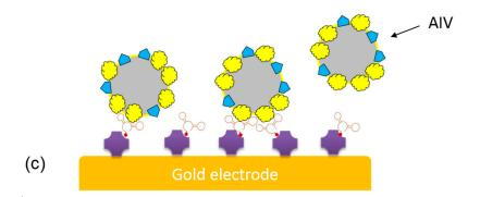
Figure S2. Design of the impedance aptasensor for the detection of AIV H5N1. (a) The microelectrode surface was modified using streptavidin; (b) The biotin-labeled aptamer was then immobilized through biotin-streptavidin binding; (c) Target AIV H5N1 was captured and the impedance was measured. After each step the flow cell was washed to remove unbound particles.
