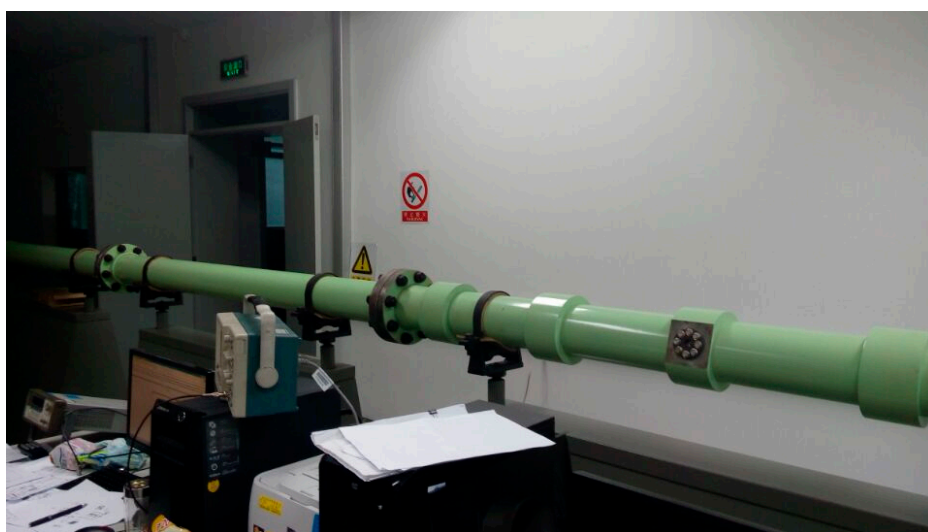
Figure 4. Shock tube calibration test.
