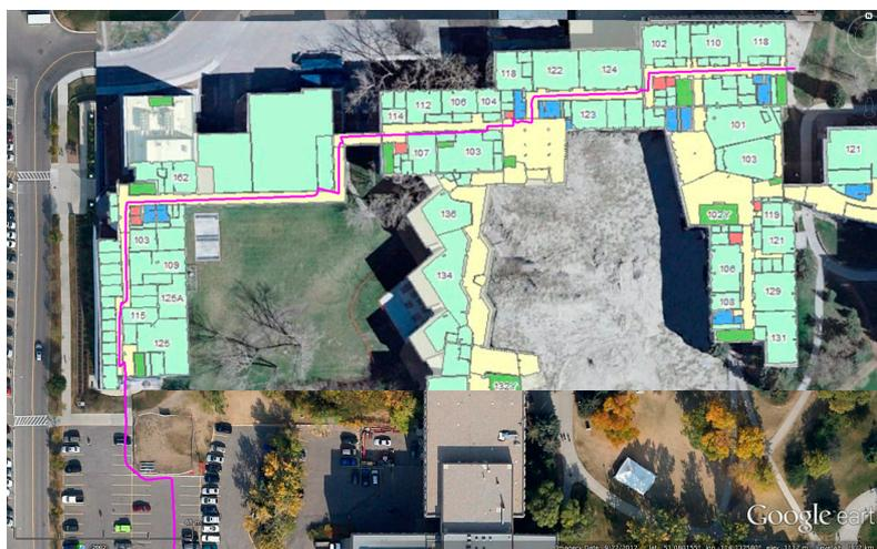
**Figure 14.** The trajectories used to generate WiFi DB in ENB.
