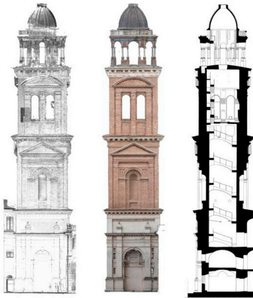
**Figure 11.** Santa Barbara bell tower. Laser scanning and photogrammetry data and a final elaboration of a vertical section obtained using both the technologies.
