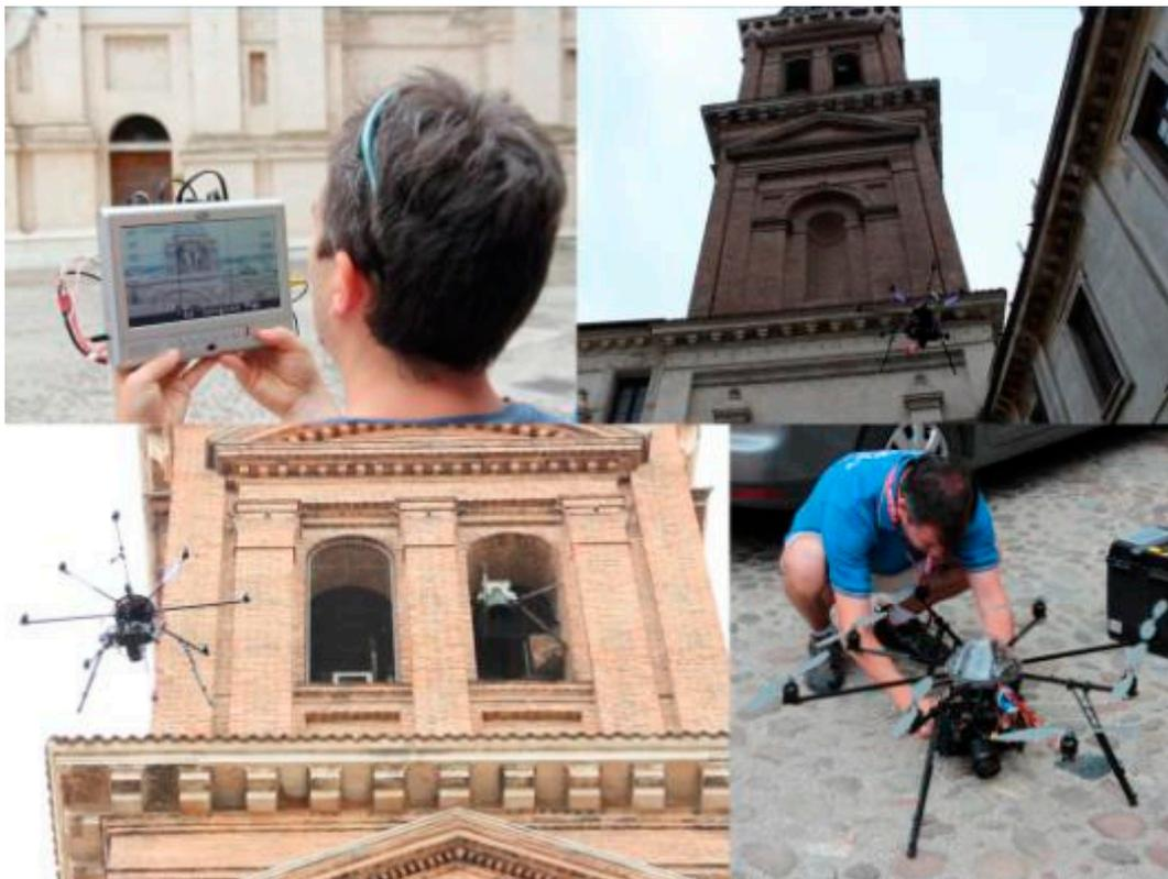
**Figure 6.** The octocopter employed for the bell tower acquisition, and the Wi-Fi camera controller.
