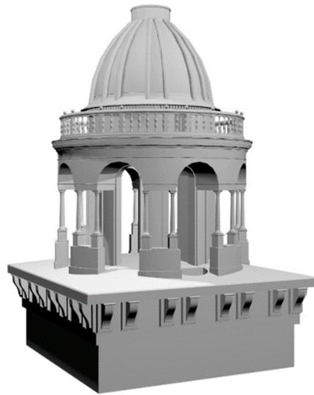
**Figure 10.** 3D model of the round temple for FEM analysis.
