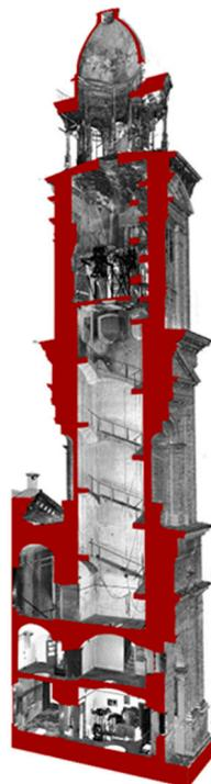
**Figure 4.** Laser scanner point clouds of interior and exterior registered in the local reference system for the elaboration of the section.
