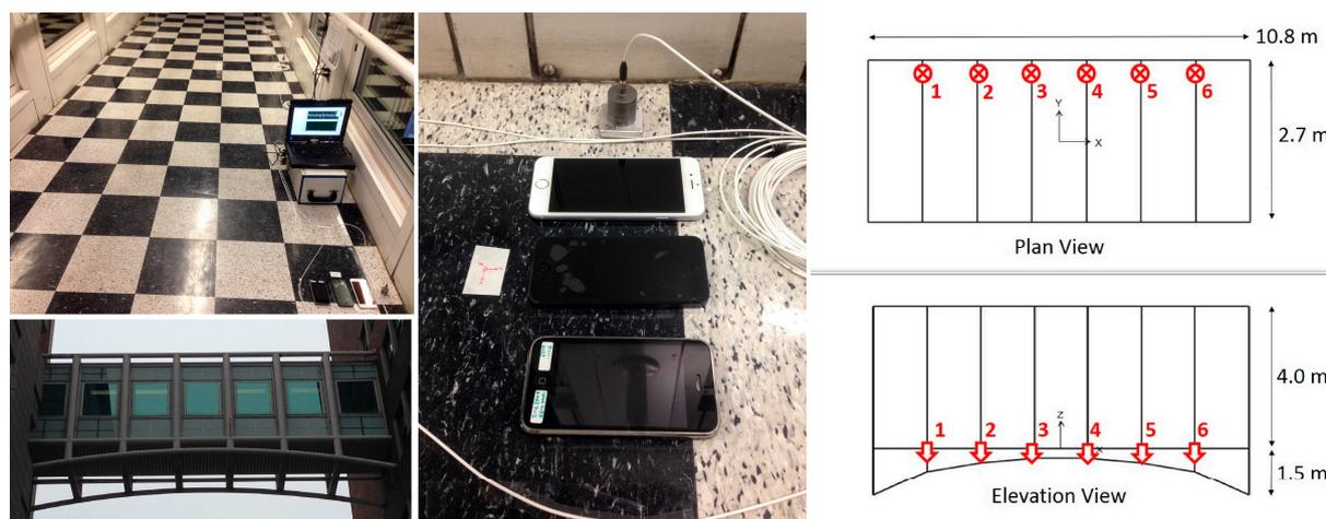
**Figure 5.** Inner and outer views, dimensions, and sensor layout of the pedestrian link bridge.
