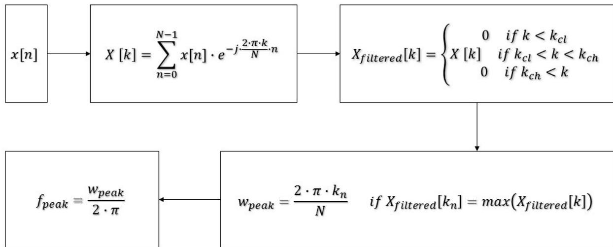
**Figure 3.** Digital signal processing operations applied on the server-side.
