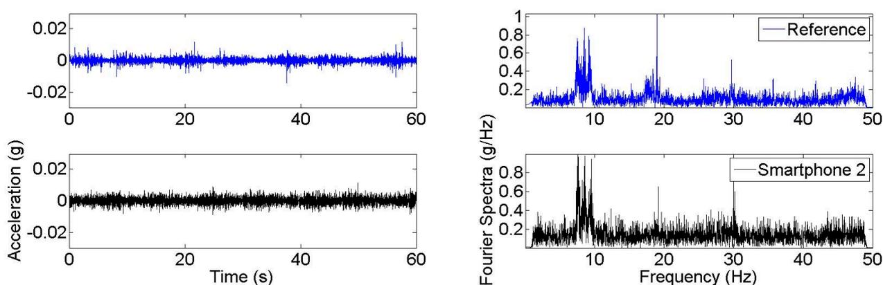
**Figure 12.** Acceleration time histories and Fourier spectra samples from pedestrian-induced vibrations.
