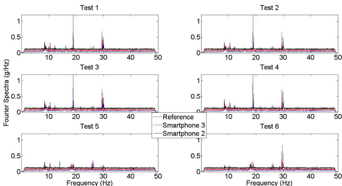
**Figure 8.** Fourier spectra from the average of 40 samples for Test 1–6.
