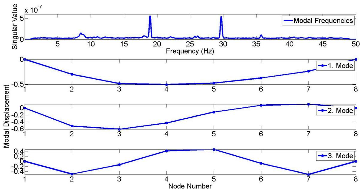
**Figure 6.** 1st, 2nd, and 3rd modal frequencies (8.46, 18.95, 29.67 Hz) and mode shapes from FDD by reference accelerometers.
