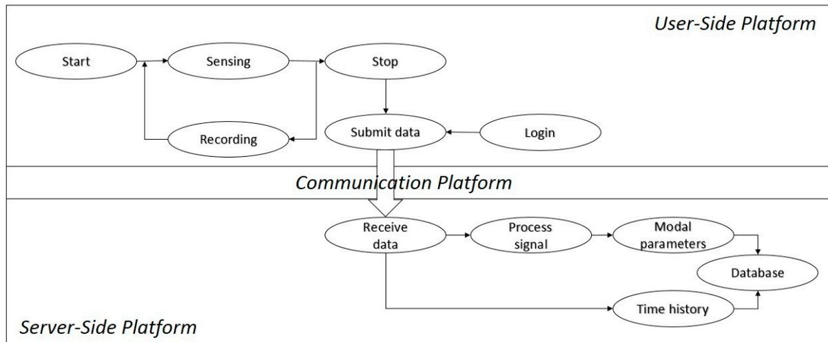
**Figure 1.** Integration scheme of system platforms.
