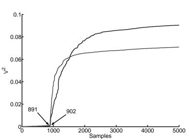
**Figure 4.** Cumulative energy of the same signals of Figure 3. Notice that the actual shift between them is only 11 samples instead of 127.
