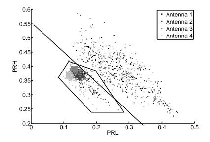
**Figure 8.** 2D mapping of all pulses from the second object considering the low frequency interval in [50, 300] MHz and the high frequency interval in [600, 1600] MHz.
