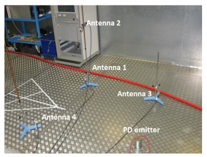
**Figure 2.** Setup in laboratory. Notice the abundance of metallic surfaces and structures around the antennas.
