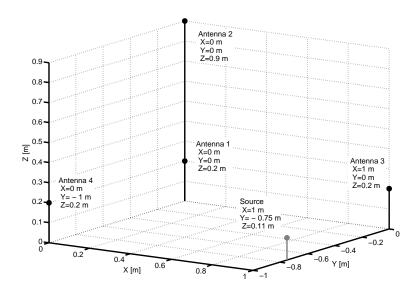
Figure 1. Antennas and first PD emitter position.
