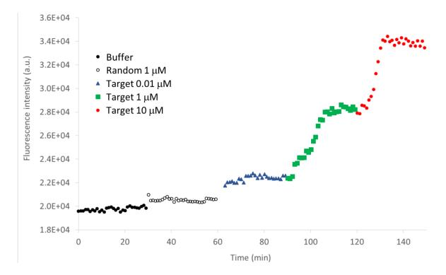
**Figure 7.** Fluorescence signal (*vs.* time) during the interaction of the MB immobilized onto the nanotip with the random sequence, and the target at different concentrations (0.01  $\mu$ M, 1  $\mu$ M and 10  $\mu$ M).
