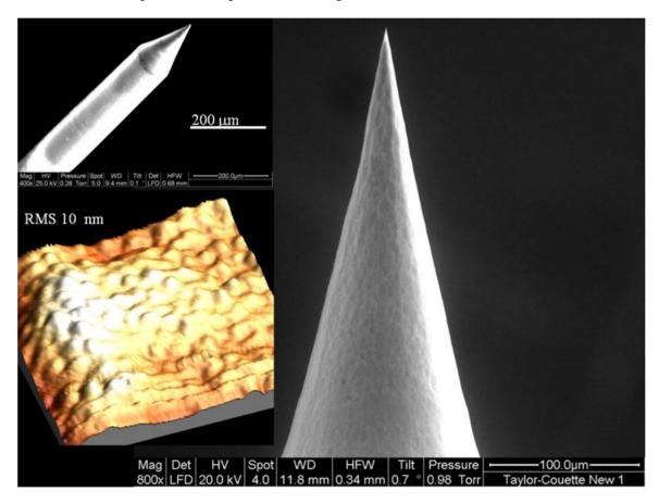
**Figure 2.** Example of a nanotip obtained using the fabrication method described in Section 2.3. In the left top a general view showing a taper length of about 200  $\mu$ m and a large cone angle (about 40 °), while in the left bottom an AFM image (10  $\mu$ m × 10  $\mu$ m) is reported, with an estimated roughness of about 10 nm. On the right panel is reported a zoom on the distal end, showing an apex angle of about 24 °.
