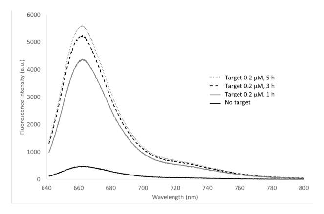
**Figure 4.** Fluorescence spectra of the molecular beacon (0.1  $\mu$ M) after incubation for 1, 3 and 5 h with the specific target 0.2  $\mu$ M.  $\lambda_{ex}$  635 nm, exposure time 1 s.
