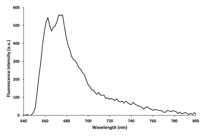
**Figure 5.** Fluorescence spectra of the linear probe immobilized onto the nanotip.  $\lambda_{ex}$  635 nm, exposure time 1 s.
