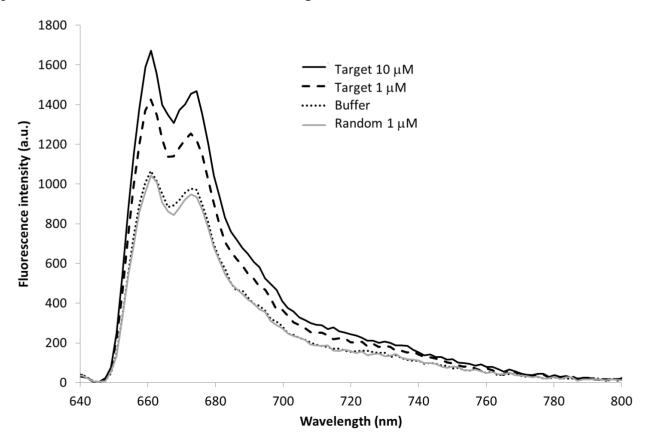
**Figure 6.** MB immobilized onto the nanotip, characterization in presence of the target (1  $\mu$ M and 10  $\mu$ M) and of the random sequence (1  $\mu$ M).  $\lambda_{ex}$  635 nm, exposure time 1 s.
