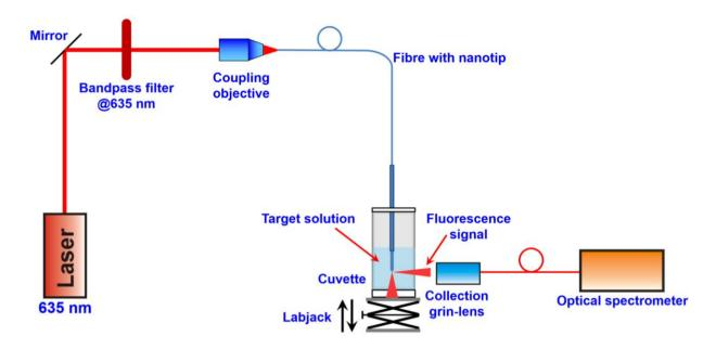
Figure 3. Optical experimental set-up.
