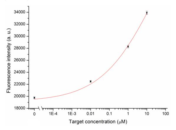
**Figure 8.** Calibration curve obtained from the interaction of the MB-coated nanotip with increasing concentrations of target.
