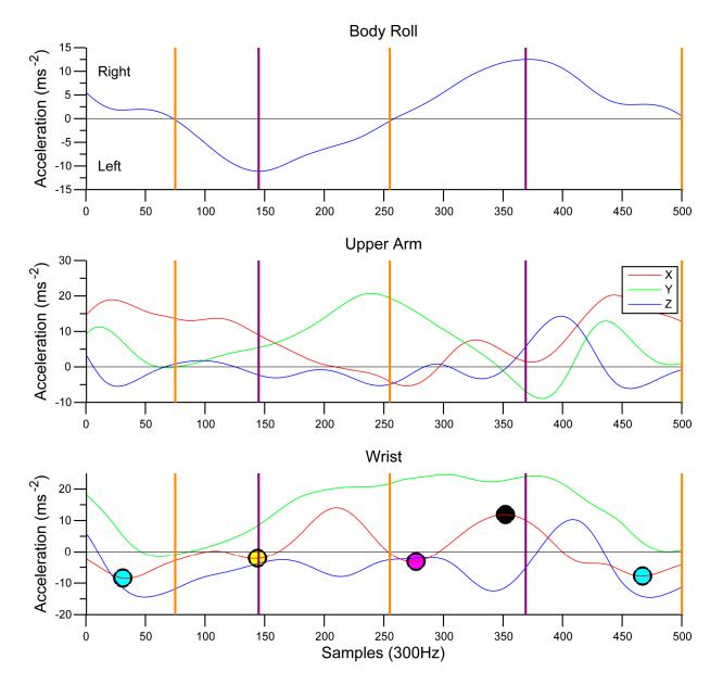
**Figure 4.** Identification process of the phases in the stroke (Swimmer R). Entry (Cyan dot), Start of Pull (Yellow dot), Start of Push (Magenta dot), Start of Recovery (Black dot). Zero Crossing Body Roll (Orange), Peak Body Roll (Purple).
