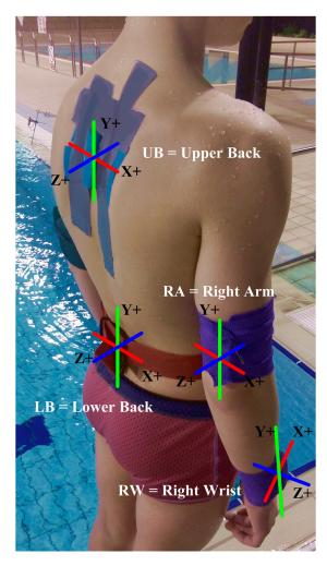
Figure 3. Device placement and attachment method and orientation.
