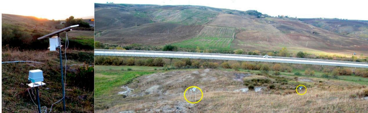
**Figure 13.** (Left) A POIS levelled and connected to the solar panel; (Right) Two sensors (yellow circles) on the toe of the monitored landslide, close to the A16 highway, near Lacedonia (Southern Italy).
