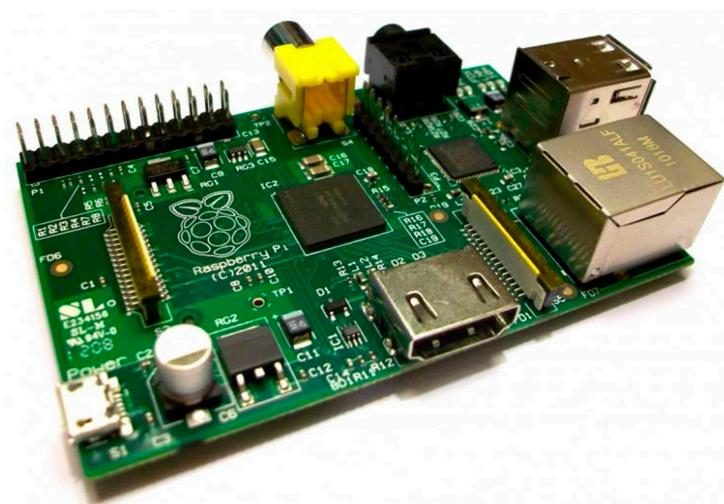
Figure 4. The Raspberry Pi computer.
