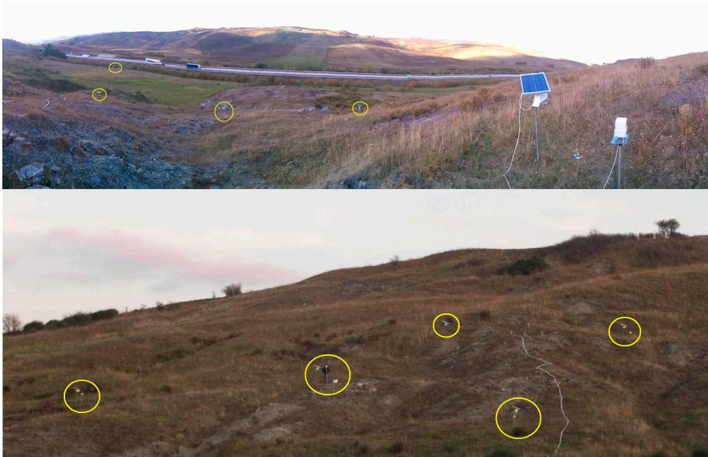
**Figure 14. (Top)** A partial view of the sensor network installed near the highway A16. The sensors are circled; the upper left sensor, out of the accumulation zone of the landslide, acts as the coordinator node; **(Bottom)** The sensor network seen from below. The cable on the right, powers a group of MEMS sensors installed in the same zone.
