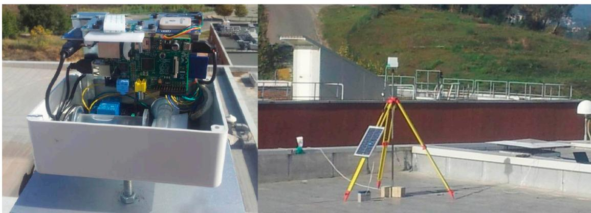
**Figure 12.** (Left) The sensor assembled; (Right) The sensor positioned on the terrace of the Geomatics Lab: the photovoltaic panel, the battery and the antenna of the GNSS permanent station are visible.
