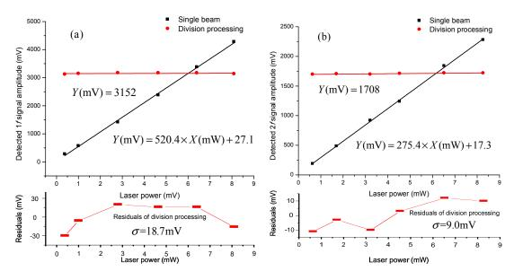
Figure 5. Test result of immunity to laser power instability. (a) is for the 1f signal and (b) is for the 2f signal.
