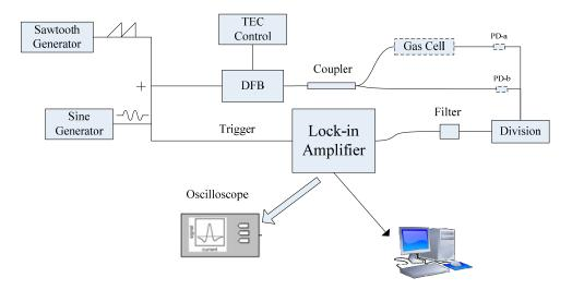
Figure 1. Schematic of WMS detection using a divider.
