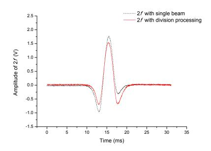
Figure 3. Comparison of 2f signals detected by the division and single beam processes.
