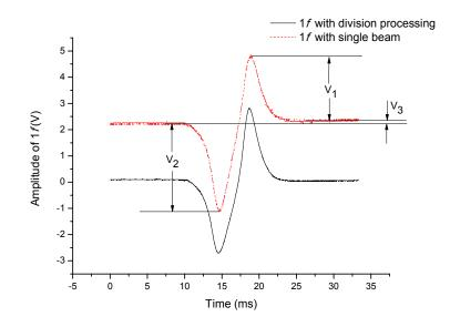
Figure 2. Comparison of 1f signals detected by the division process and single beam.
