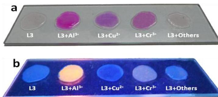
**Figure 11.** Photographs of ligand doped PVC polymeric thin films under visible (a) and fluorescent light (b).
