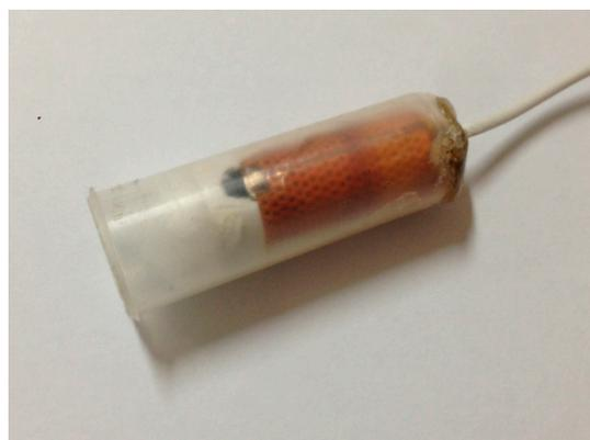
**Figure 3.** Pulse sensor.
