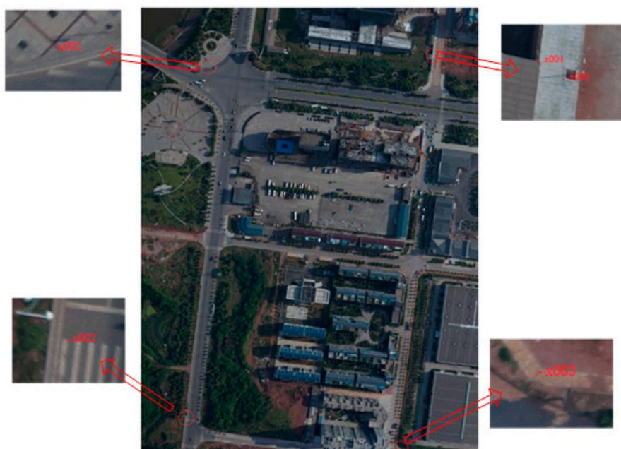
**Figure 15.** A slice of ground control points.
