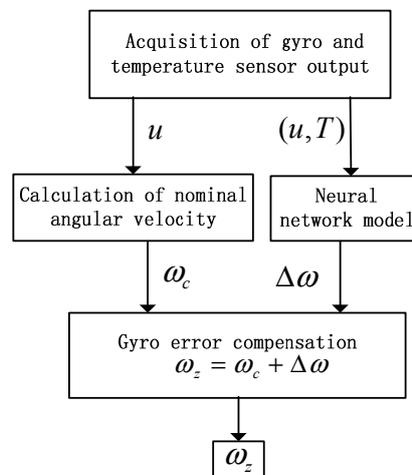
**Figure 4.** The flow of gyro angular velocity error compensation.
