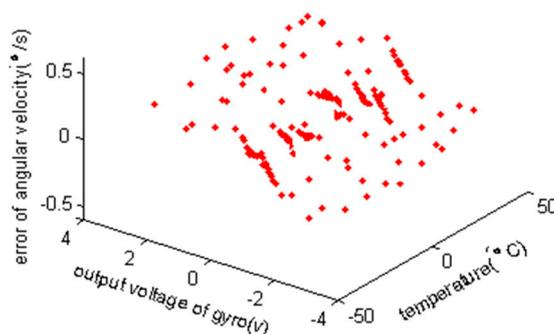
**Figure 12.** The angular velocity error of the verification data after compensation.
