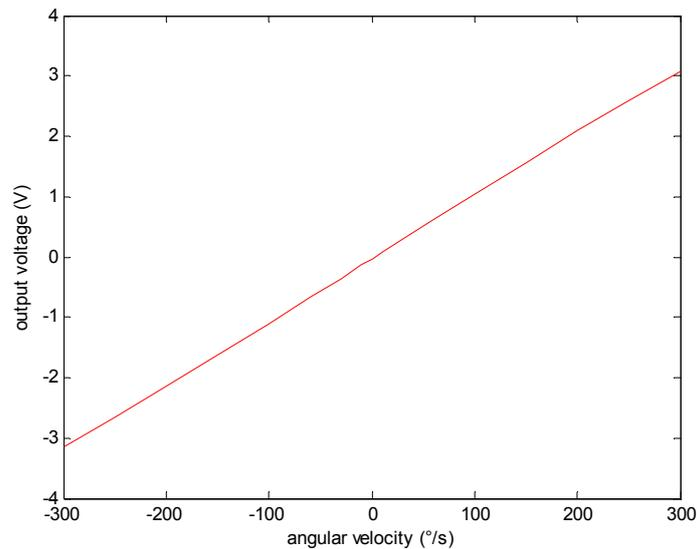
**Figure 6.** The relationship between output voltage and angular velocity.
