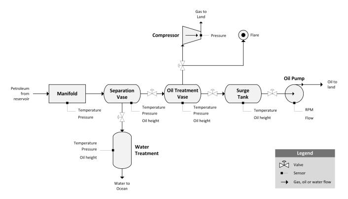
**Figure 1.** Oil platform process plant work-flow.
