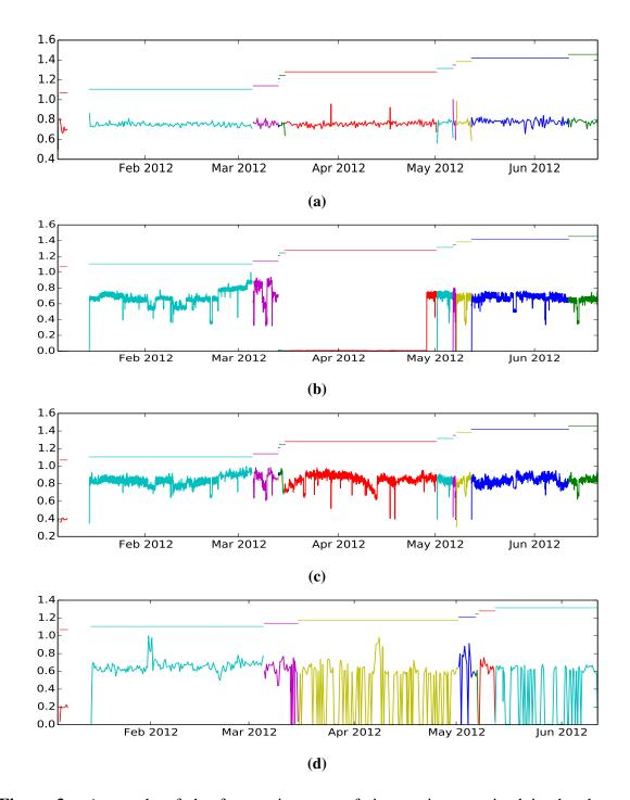
**Figure 3.** A sample of the four main types of time series contained in the dataset. We have marked with color changes the moments in which the machine was switched on/off. (a) Homogeneous time series; (b) unstable/noisy time series; (c) multi-modal series; (d) highly unstable time series, probably caused by faulty sensors.
