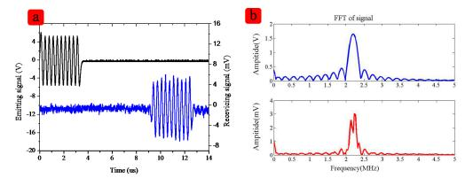
**Figure 7.** The response of one typical array element. (**a**) shows the emitting signal and the receiving signal; (**b**) shows the FFT of the signals, the spectrum signal.
