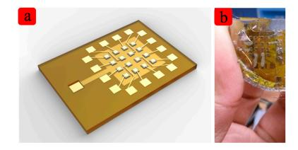
**Figure 1.** (a) shows the schematic diagram of the FpMUT; (b) The device is packaged with PDMS and it is flexible, stretchable and causes no harm to humans.
