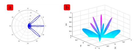
Figure 3. The directivity simulation results with the Matlab software. The distance between two elements in about 1.5 times the wavelength (a) shows the 2-dimensional figure and (b) shows the 3-dimensional result.
