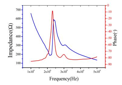
Figure 5. The experimental results of impedance and phase.
