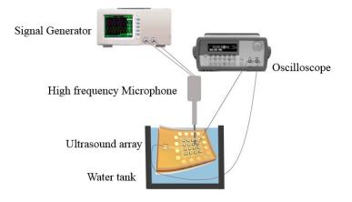
**Figure 6.** The schematic diagram of the test. The whole device tested in the water tank without any waterproof material.
