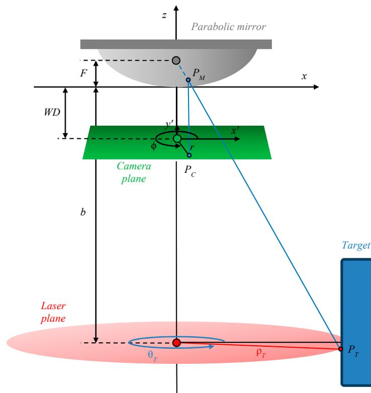
**Figure 2.** Schematic view of the proposed setup. The final goal of the analytical model is the translation of the known coordinates  $(r_C, \phi_C)$ , recovered on the camera plane, in world coordinates  $(\rho_T, \theta_T, z_T)$ , having origin in the mirror vertex.
