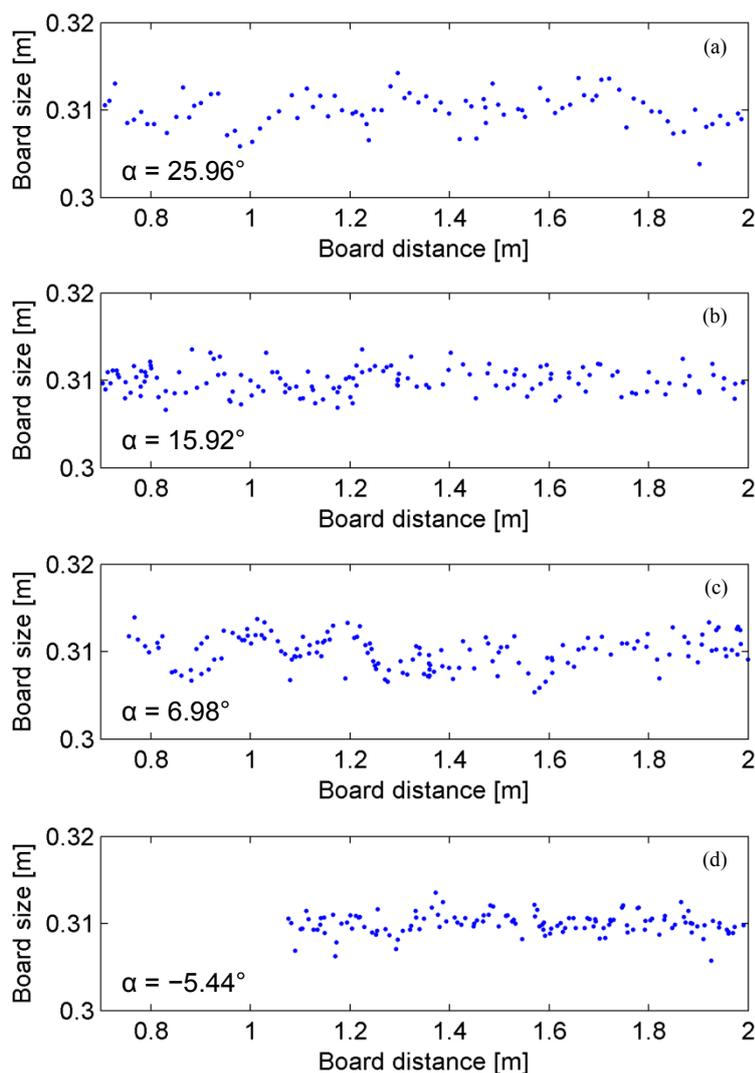
**Figure 12.** Estimation of the size of the sample board as a function of the distance of the target from the light sources. Measurements have been performed changing the direction of the radial shifts, accordingly with the axis defined by the angle  $\alpha$ , referred to the ground plane: (a)  $\alpha = 25.96^\circ$ ; (b)  $\alpha = 15.92^\circ$ ; (c)  $\alpha = 6.98^\circ$ ; (d)  $\alpha = -5.44^\circ$ .
