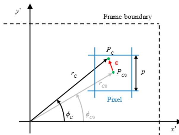
**Figure 3.** Error components related to the quantization of the image plane due to the finite area of pixels. Each pixel of the plane is square and has side equal to the pixel pitch  $p$ .
