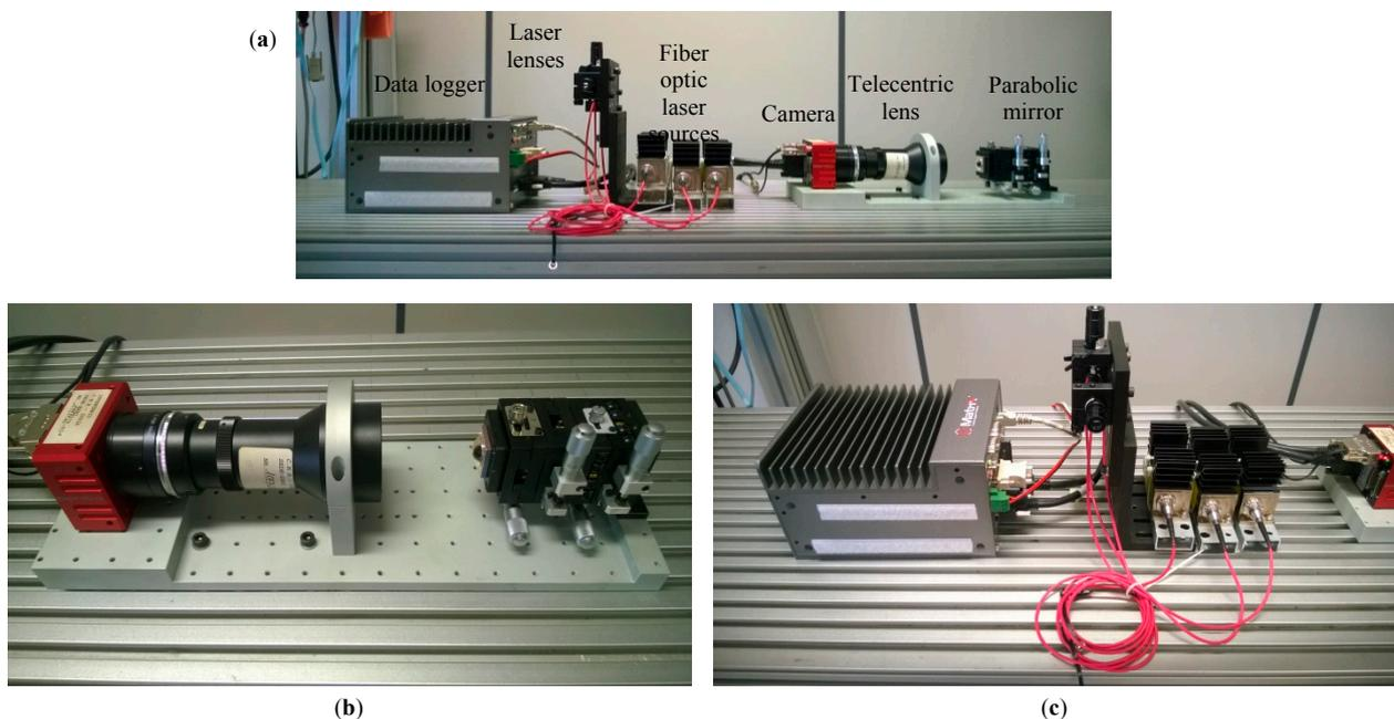
**Figure 4.** Picture of the actual prototype: (a) Overall setup; (b) Optical receiver made of the parabolic mirror and the lens-camera set; (c) Laser sources and lenses and data logger connected to the camera.
