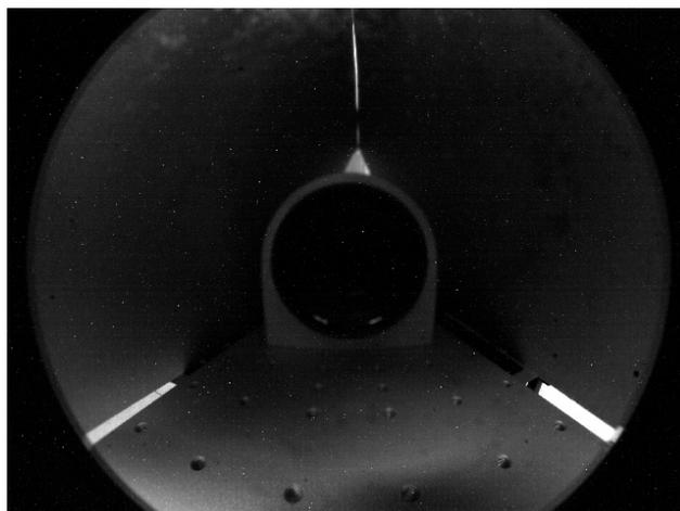
**Figure 7.** Example of frame captured by the camera for the estimation of the mirror position in the image plane.
