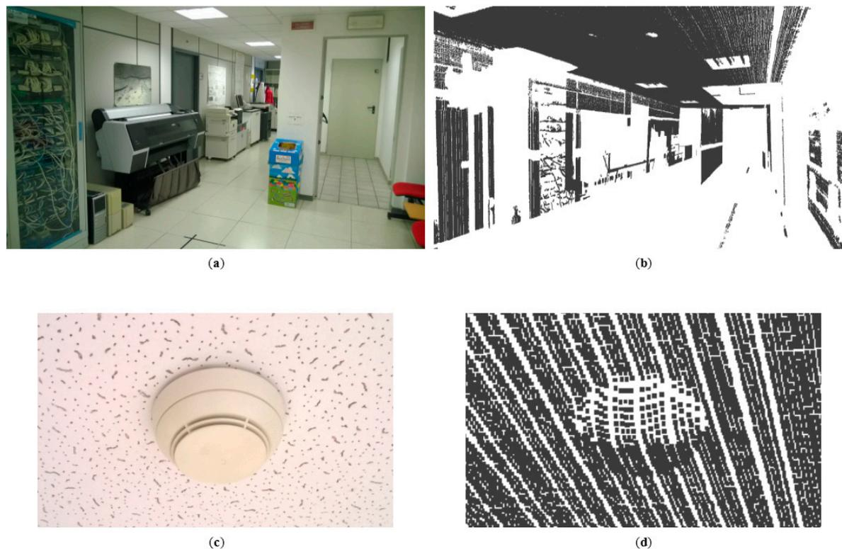
**Figure 14.** (a) Acquired corridor and (b) corresponding 3D reconstruction; (c) picture of a particular object with maximum size of 10 cm and (d) corresponding 3D model.
