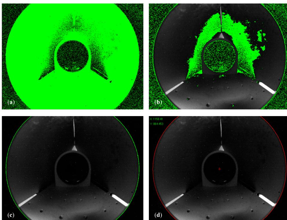
**Figure 8.** Image processing steps for the determination of the mirror position in the camera plane. (a) Threshold image; (b) Boundaries extracted from the threshold regions of high intensity; (c) Start image and corresponding fitting ellipse (in green); (d) Final results with the estimation of the center coordinates (red cross).
