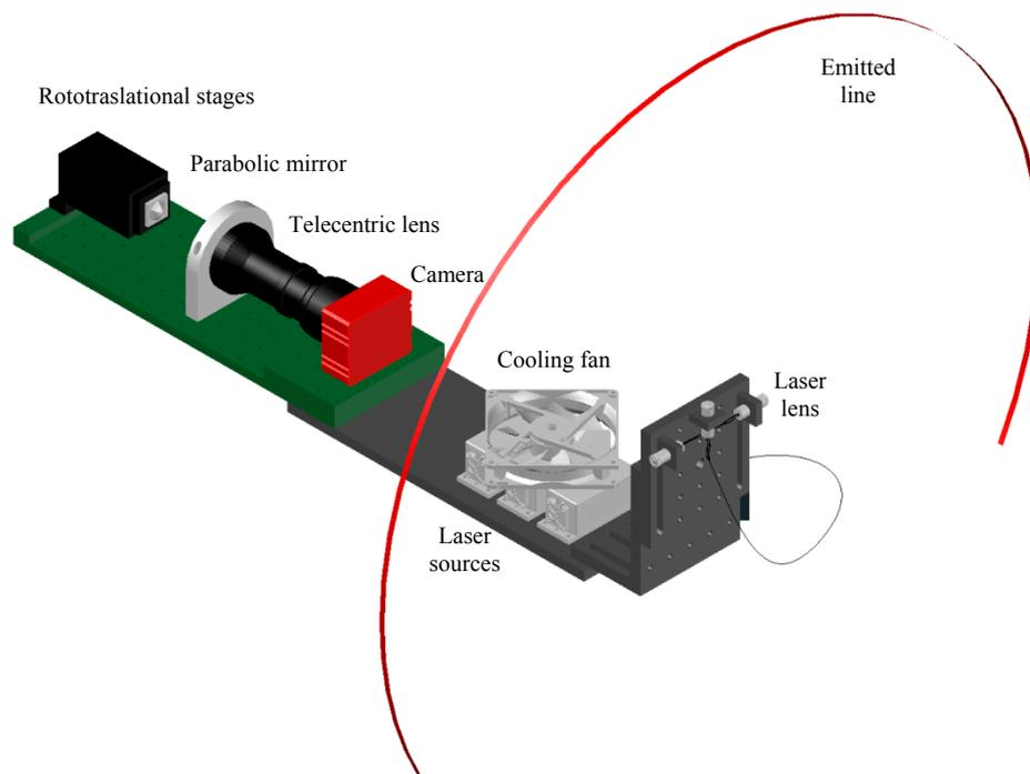
**Figure 1.** Sketch of the presented laser profilometer. Note the parabolic mirror is mounted onto micrometric rototranslational stages, whereas the camera is fastened on the metallic stand. Lasers are placed across from the parabolic mirror, behind the camera.
