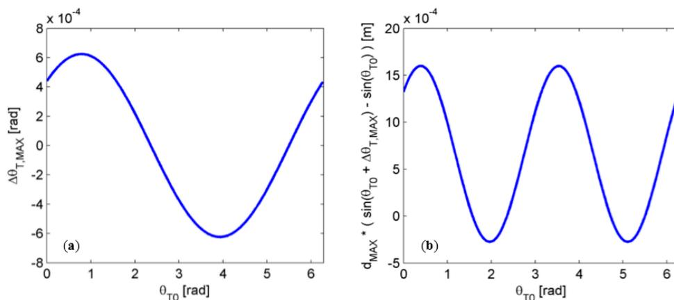
**Figure 6.** **(a)** Angular component of the maximum measurement error at  $d_{MAX} = 3$  m as a function of the estimated angle  $\theta_{T0}$ ; **(b)** Maximum estimated shift, due to the presence of angular uncertainty  $\Delta\theta_{T,MAX}$ , in the computation of the  $y$ -coordinate of the point  $P_C$  at  $d_{MAX}$  equal to 3 m.
