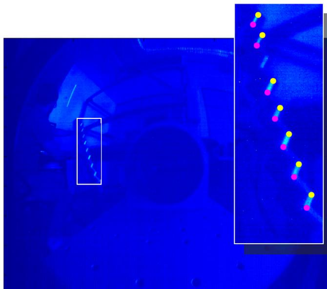
**Figure 9.** Example of a frame captured by the camera during the setup calibration. The laser line illuminates a target of completely known geometry. The inset highlights the extracted points belonging to the structure edges, whose distance corresponds to the thickness of the wood strips.
