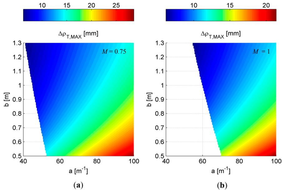
**Figure 5.** Maximum errors  $\Delta\rho_{T,MAX}$  at  $d_{MAX} = 3$  m as a function of the mirror curvature and the baseline, computed for magnification equal to: **(a)** 0.75; **(b)** 1. Regions where the laser incidence is out of the camera FoV are displayed in white.
