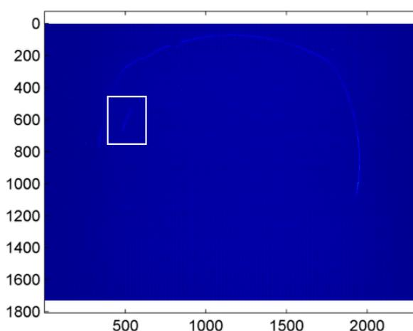
**Figure 10.** Example of frame acquired by the camera for testing the sensor accuracy. The rectangle encloses the laser line impinging on the board.
