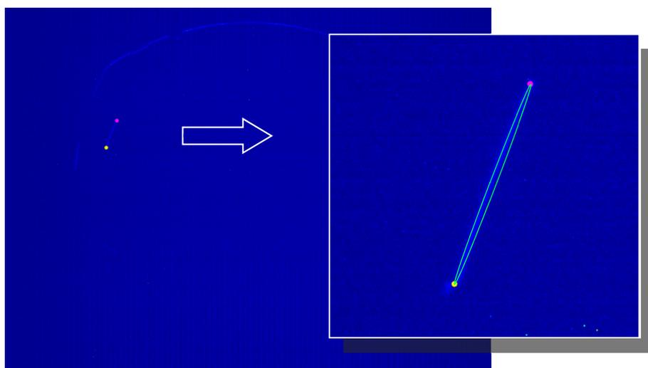
**Figure 11.** Results of the edge extraction algorithm used for the detection of the board sizes. The inset shows a magnified view of the extracted points; the green line identifies the fitting ellipse.
