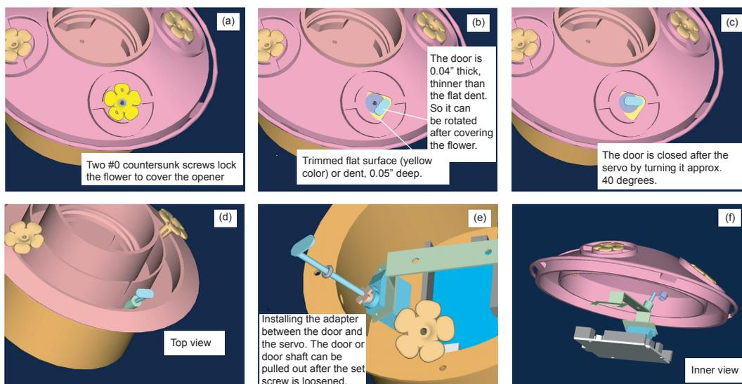
**Figure 7.** Computer aided design models of installing custom feeder opener on an off-the-shelf hummingbird feeder. The main steps include (a) modifying the flower opening; (b) resurfacing the area beneath the flower opening; (c) and (d) installing the servo operated door; (e) connecting the door to the servo motor, and (f) installing the servo motor underneath the feeder.
