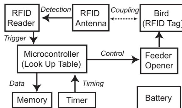
Figure 2. System schematic of the smart feeder system.
