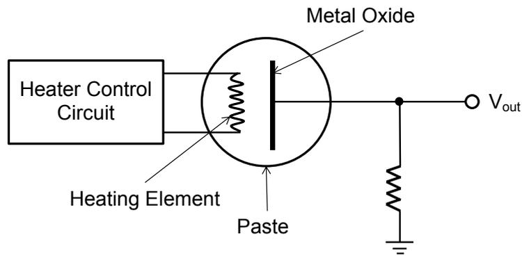
Figure 2. Bead-type sensor.
