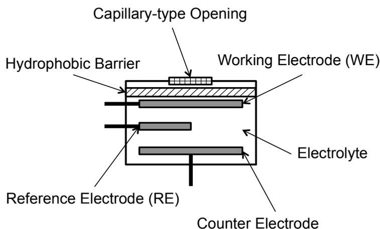
Figure 4. Basic Electrochemical Sensor.
