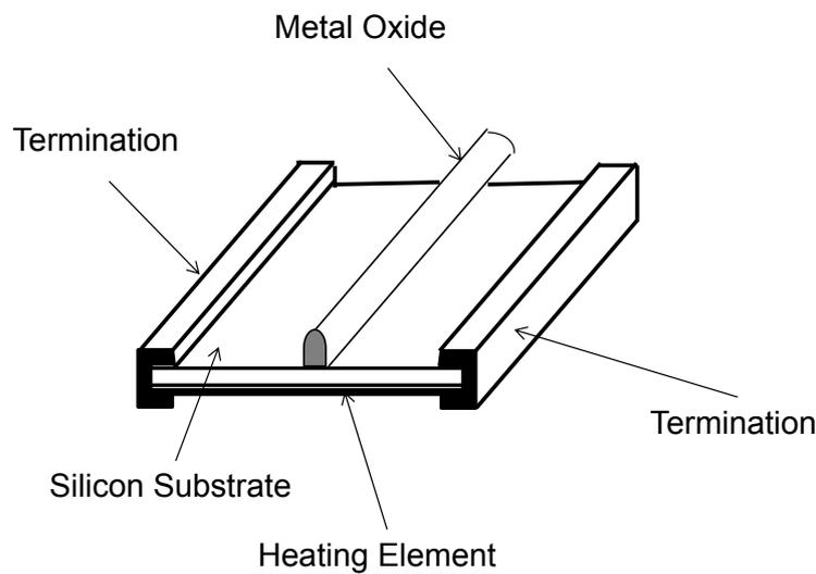
Figure 3. Chip-type Sensor.
