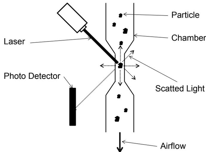
Figure 5. Basic Light Scattering Particle Counter.
