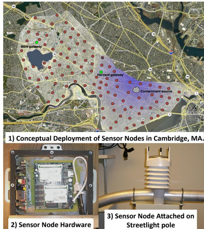
**Figure 8.** Example of the SSN system architecture and prototype. Red dots are the sensor nodes. Green dots are the gateways that forwarding the acquired data to the Contaminant Source. Figures are adapted from [101].
