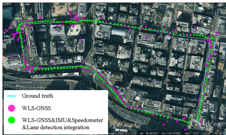
(a) WLS-GNSS and WLS-GNSS based integration
