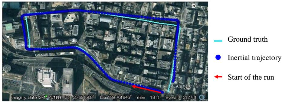
Figure 8. Drift effect of IMU sensor.
