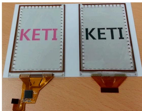
**Figure 4.** Image of the fabricated SWCNT based force sensing touchscreen composed of substrates of transparent glass and PET film and a force sensing inner layer of elastic silicone inserted between the two electrodes.
