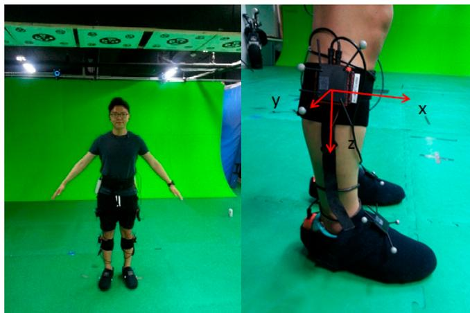
Figure 13. Experimental setting to compare the results of the proposed algorithm with the Vicon setup.
