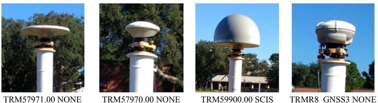
**Figure 5.** Antennas used in Phase 1 [18].
