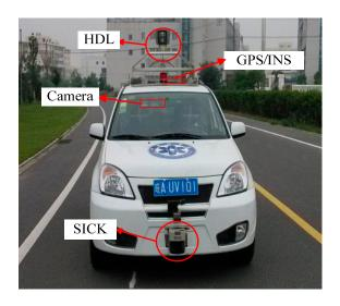
Figure 1. The autonomous vehicle named "Intelligent Pioneer".
