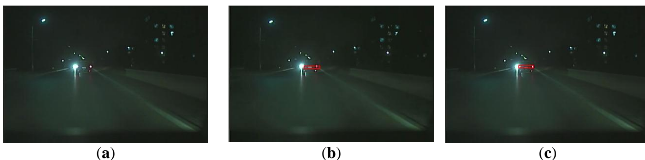
Figure 13. Comparison of vehicle detection results (case 4): (a) Result using the global rule-based algorithm; (b) Result using Kalman tracking-based global algorithm; (c) Result using the proposed algorithm.
