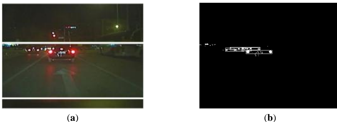
Figure 5. Result of taillight pairing based on the similarity analysis: (a) Original image; (b) Result of taillight pairing.
