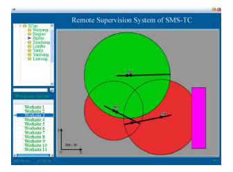
After login, the user can select a city and a specific building site via a menu. All the registered tower cranes can be found with the project information, tower crane configuration, real-time data, real-time video signals as well as the historical data, alarm times and so on. The statistical information can be generated to facilitate supervision.
