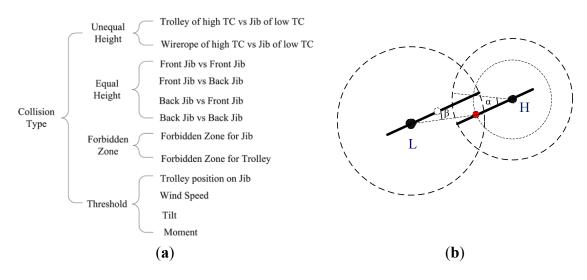
If  $T_H > h_L$ , there is no chance for the collision of two tower cranes.
