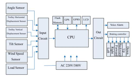
Figure 7. Functional block diagram of safety management system for tower crane (TC-STE).
