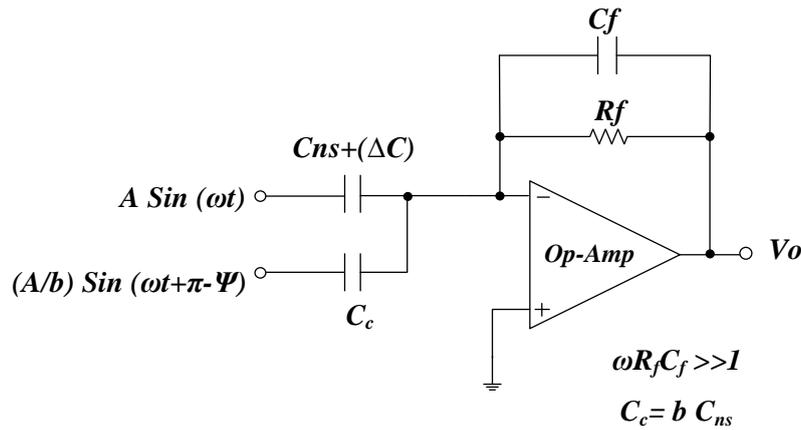
**Figure 4.** Circuit to generate compensating driving signals.
