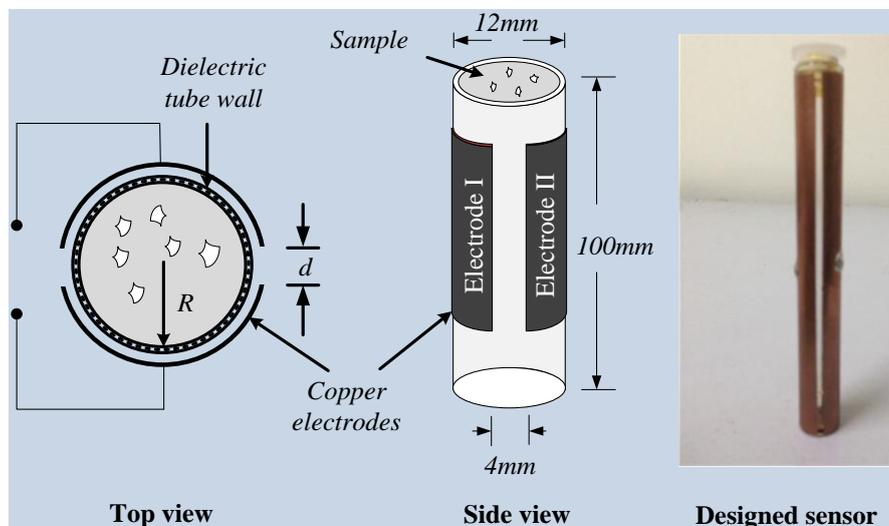
The capacitance of the sensor depends on the dielectric permittivity of medium between the pair of electrodes. The actual capacitance ( $C_a$ ) due to crude oil sample is in series with glass tube wall capacitance ( $C_w$ ). Therefore the total capacitance ( $C_t$ ) of the sensor can be expressed as:
