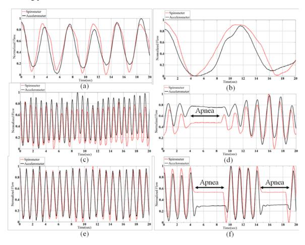
**Figure 7.** Average correlation between spirometer and accelerometer signals and the standard deviations for five different disorders.
