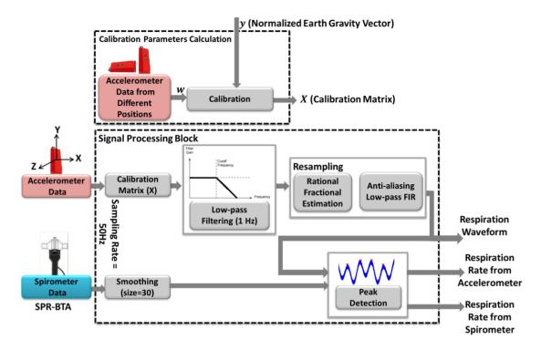
**Figure 2.** Signal processing of respiration rate analysis.
