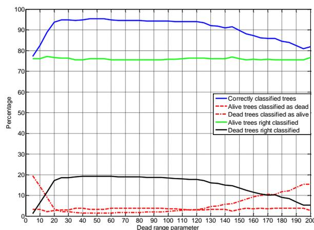
Similar to that of the LIDAR sensor, the evaluation range of the dead range parameter was from 12.7 to 508 cm steps of 5 encoder values. Considering the validation tables obtained for each dead range value (Figure 9) and the tree classification established by the LIDAR sensor, a parameter value of 50 was selected.
