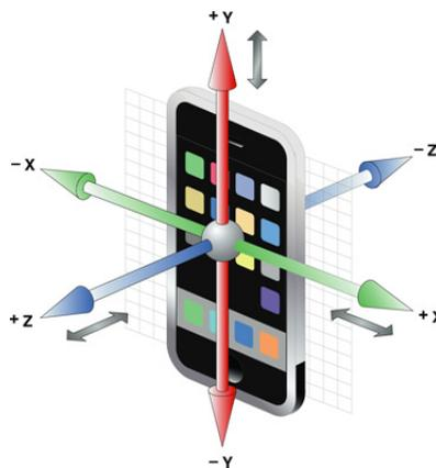
The mobile device is located on the central part of the waist, corresponding to the body's center of gravity. For maintaining the acceleration axis, the device is fixed in a special phone case attached to the user's belt. The process is split into three main stages. The system starts to receive data from the accelerometer and calculates the overall acceleration value  $Act$ :
