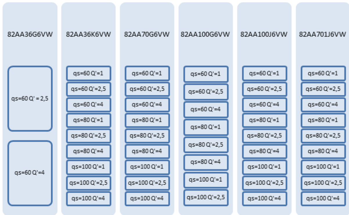
Figure 2. Grinding wheels and grinding conditions of the experimental database for training and testing the ANN-based sensors.
