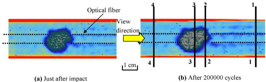
**Figure 5.** Optical micrograph of the Section 2-2 showing the positions of the fiber sensor and the extent of post-impact damage (a) just after impact; (b) after 200,000 cycles.
