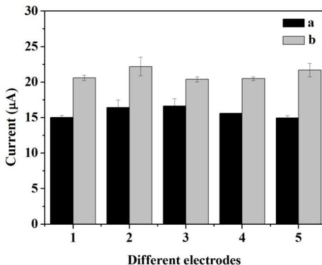
**Figure 10.** The long-term stability of the response of (a) CNFs/Lac/Nafion/GCE and (b) Cu/CNFs/Lac/Nafion/GCE. Conditions: scan rate 100 mV s<sup>-1</sup>, pH 5.5(a), pH 6.0 (b). The error bars indicate the standard error for three measurements with the same electrode.
