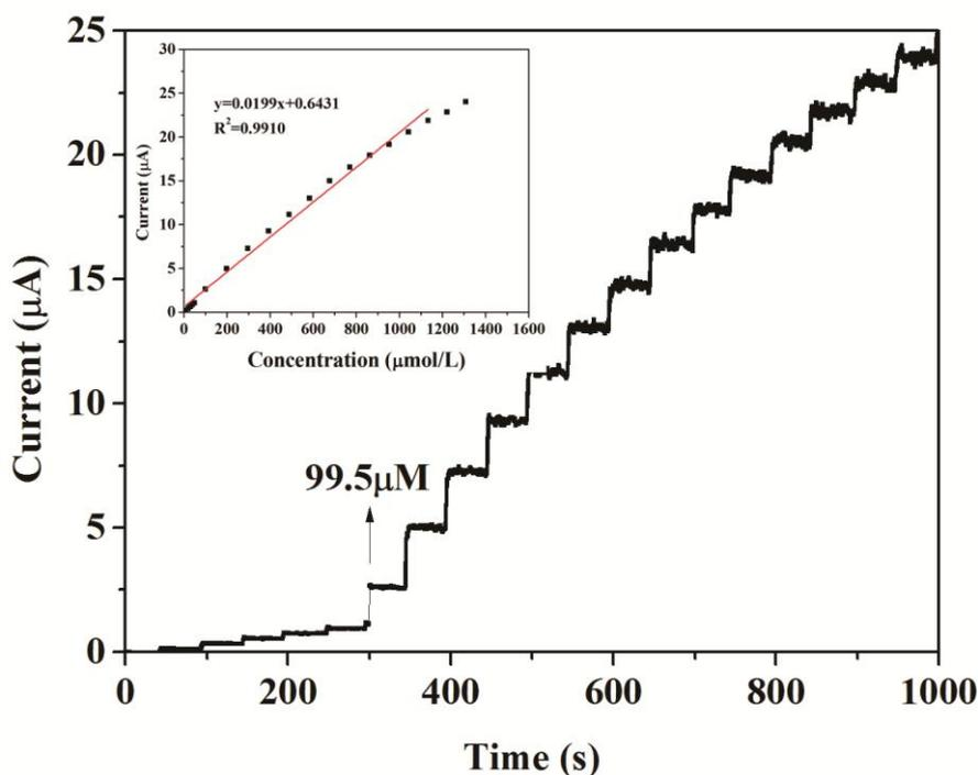
**Figure 8.** Current-time curve of Cu/CNFs/Lac/Nafion/GCE with successive addition of catechol in 0.10 M, pH 6.0, acetate buffer solutions at operating potential of +0.5 V(vs. Ag/AgCl). Inset: calibration plot illustrating the linear electrode response to catechol addition.
